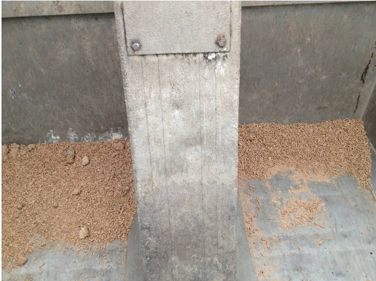
Figure 2 Picture of PIG Pellets Placed into Dump Truck Prior to Liner Installation
