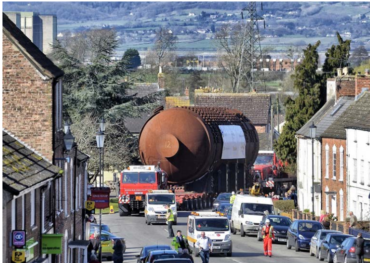
Fig. 2. 300 Mg Boiler during the transport to the export harbor in UK.
