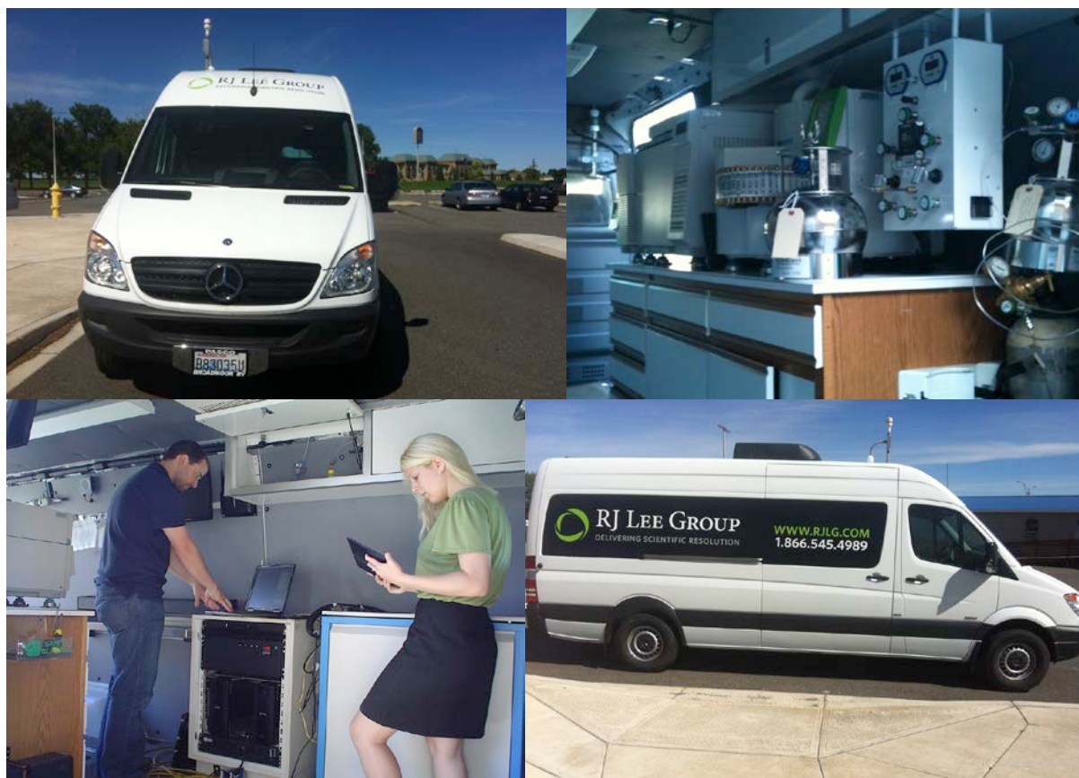
Fig. 2. The Mobile Organic Monitoring Lab featuring a Proton Transfer Reaction Mass Spectrometer (lower left) and a GC-MS with summa can and TDU tube capabilities.
