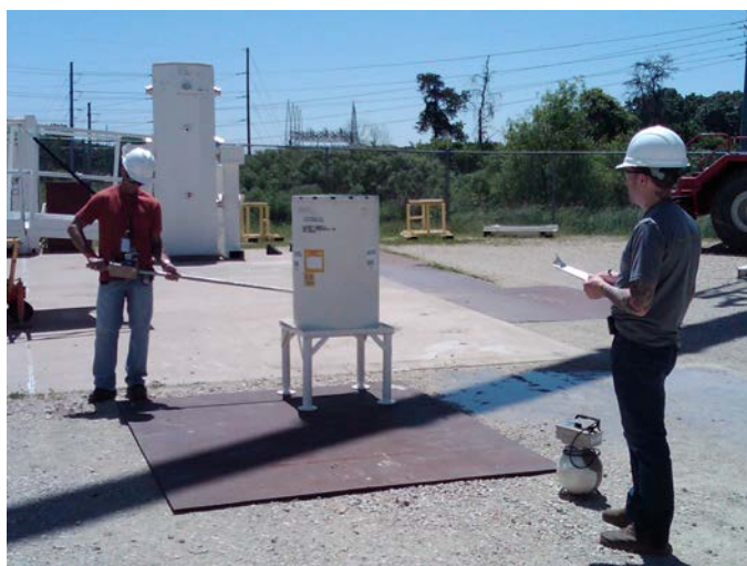
Fig. 3 – Argonne National Laboratory Rad Con Technicians taking beta, gamma surface dose rate measurements
