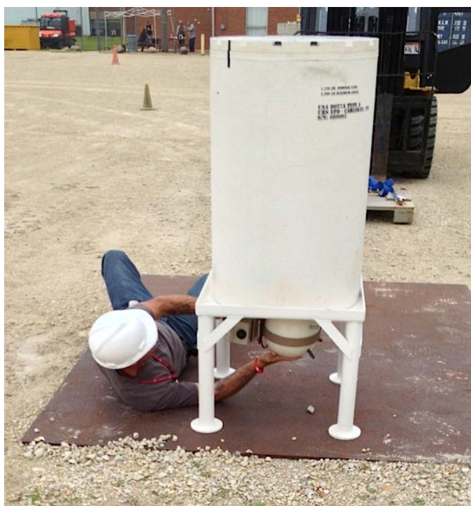
Fig. 4 – Taking neutron surface dose rate measurements on the bottom of the shielded container
