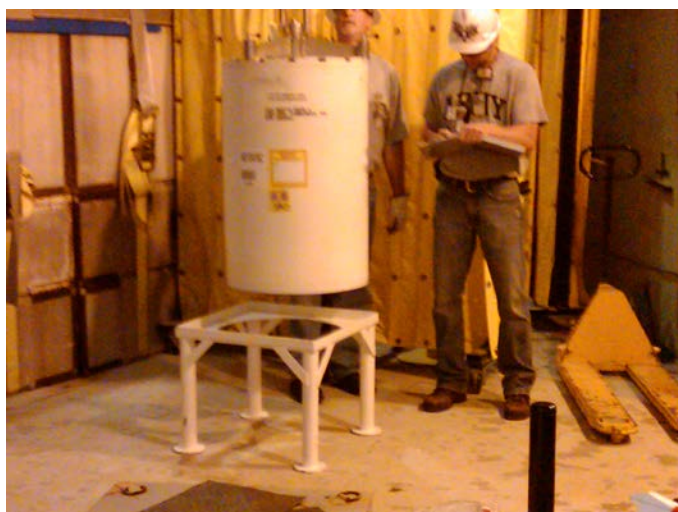
Fig 2 – Central Characterization Program Mobile Loading Team finishing closure of the shielded container prior to measurement
