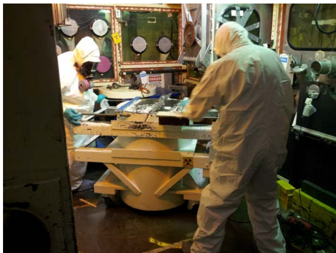
Fig. 6 – Argonne Hot Cell Technicians closing the 30 gallon drum lid that contains 2 -7 gallon cans in a sealed pouch. The 30 gallon drum is in a shielded Gated Cask (photo courtesy DOE/Argonne).
