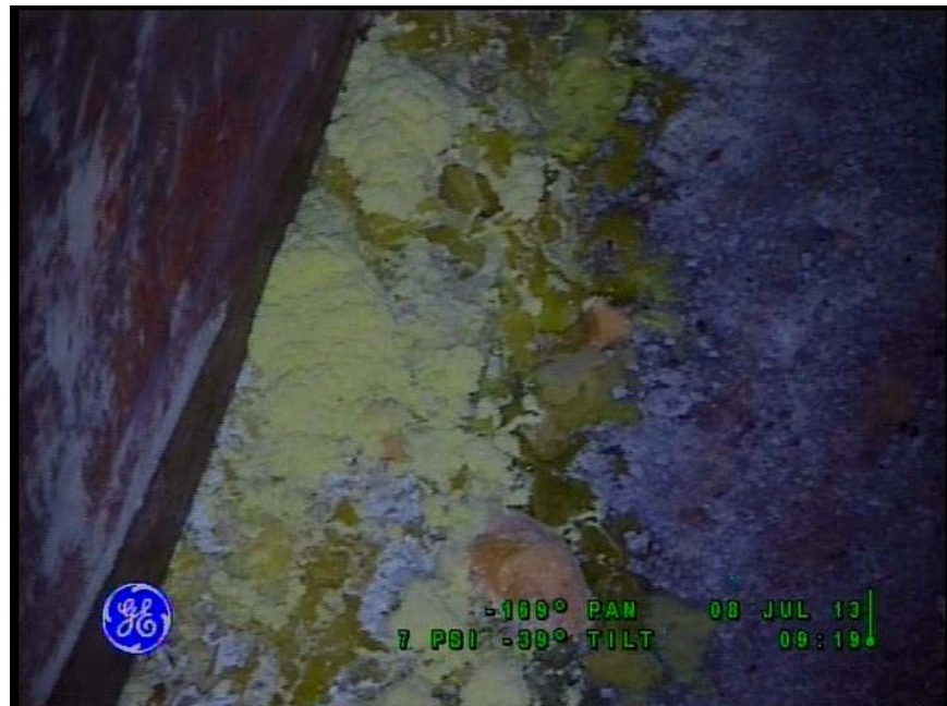
Figure 12 – 241-AY-102 Waste in the Annulus near Riser 83 (July 2013)
