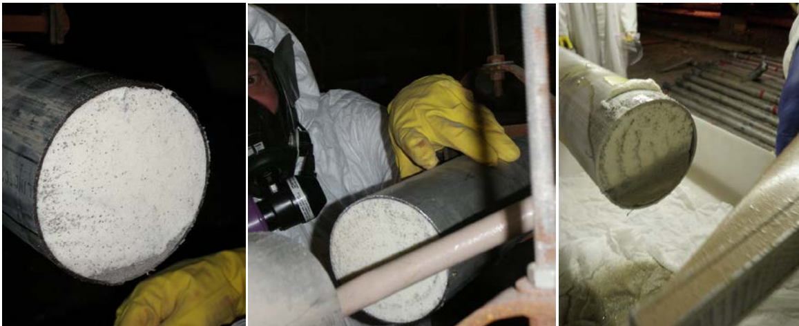
Figure 5 Examples of cut drain lines with expanding foam inside
