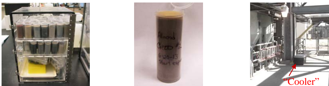
Fig. 1. Laboratory Curing Container (left); Cast Stone Sample After Curing for 30 Days Prior to Exposure Testing (center), Outdoor Exposure Container (right).
