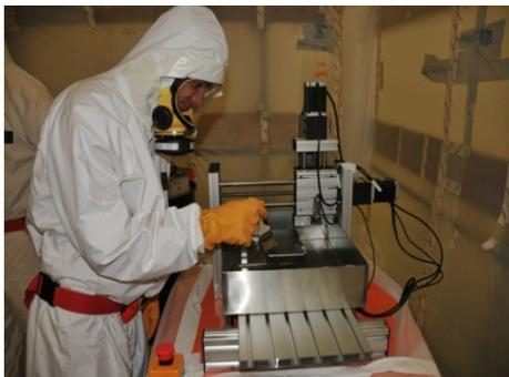
Figure 3 Bench top milling machine
