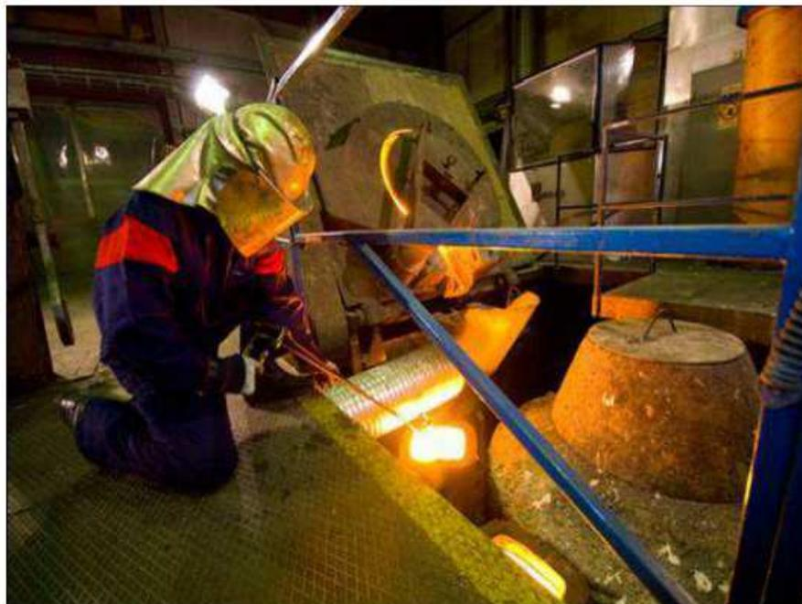
Fig.1. Induction furnace at Studsvik for melting ingots of contaminated metallic low level waste.
