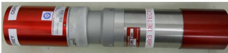
Figure 1. Stabilized 2x2 inch CeBr3 detector. The right, red section contains the scintillator crystal, and the left end is a digital tube base and multi-channel analyzer. The total overall length is approximately 33 cm.
