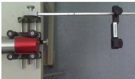
Figure 3. ISOCS characterization measurement setup with a source at 30 cm from the endcap of the CeBr3 probe. The source holder is on the right-hand side where the Am-241 / Eu-152 source is kept.
