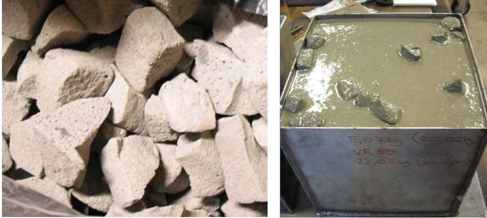
Fig. 3. Foam glass, left: material structure, right: foam glass lifted to surface during laboratory tests
