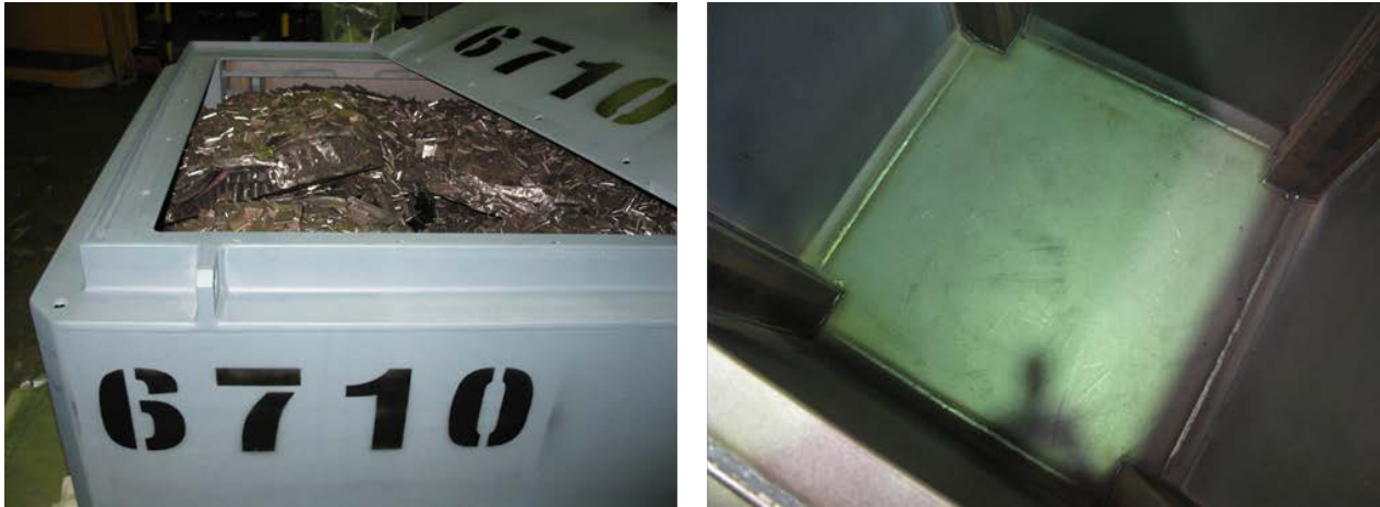
Fig. 2. Steel container, left: exterior of a loaded container before final conditioning, right: interior of container
