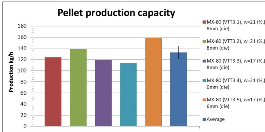
Fig. 6. Extrusion pellet production capacity of the medium size press.
