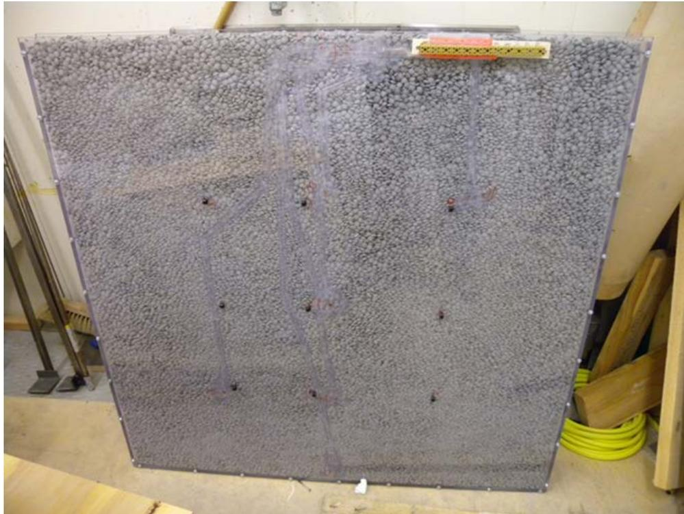
Fig. 5. A polycarbonate bentonite pellet testing mold simulating a 50 mm gap.
