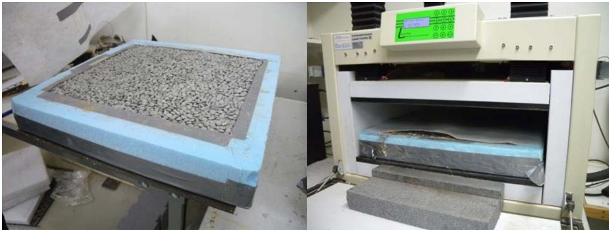
Fig. 3. Thermal conductivity measurement of the bentonite pellets with heat flow meter method.
