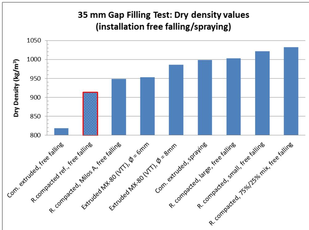
Fig. 7. Pellet dry density values from the gap filling tests.
