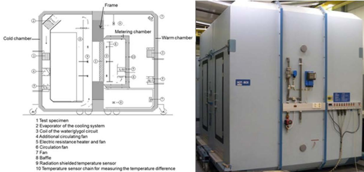
Fig. 4. Schematic arrangement of the Hot Box device.
