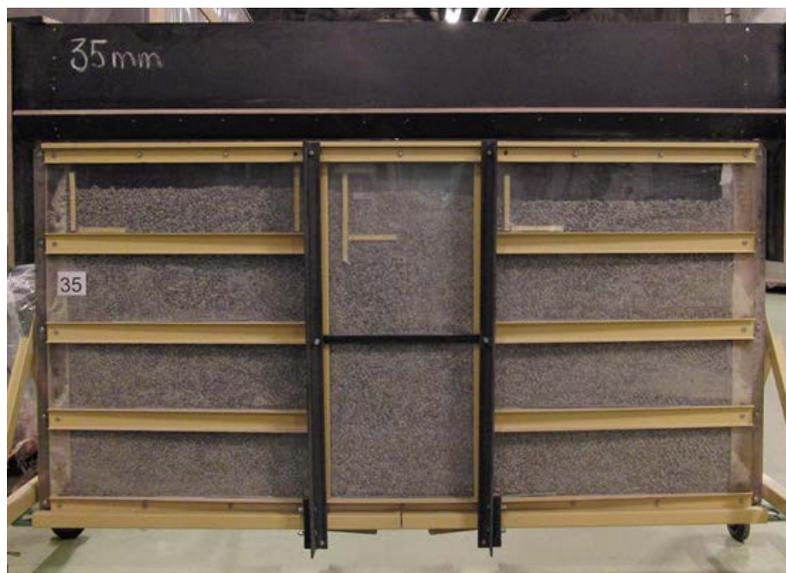
Fig. 2. The 35 mm gap filling test equipment filled with pellets.
