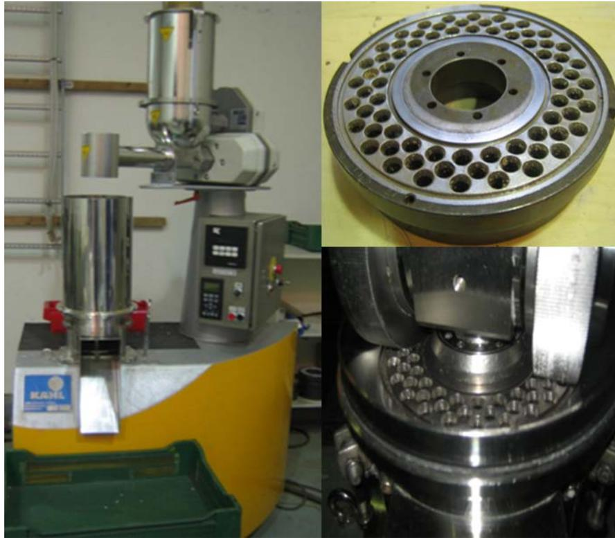
Fig.1. VTT's small pellet extrusion machine (left). Extrusion machine details: Pellet extrusion die (upper right) die and collar wheels (lower right).
