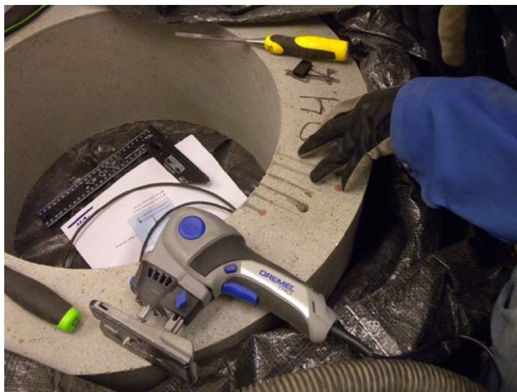
Fig. 8. The cutting and routing work of the bentonite block for the instrumentation.
