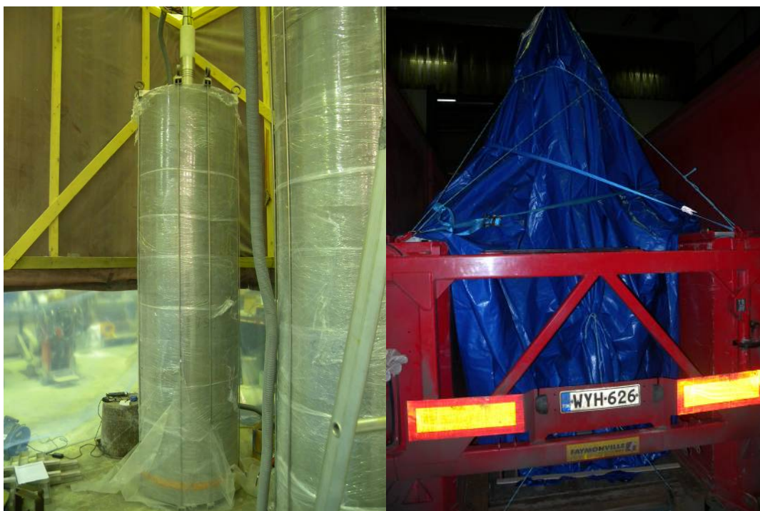
Fig. 9. Bentonite block stacks in protection tent and stacks installed in trailer for transport.
