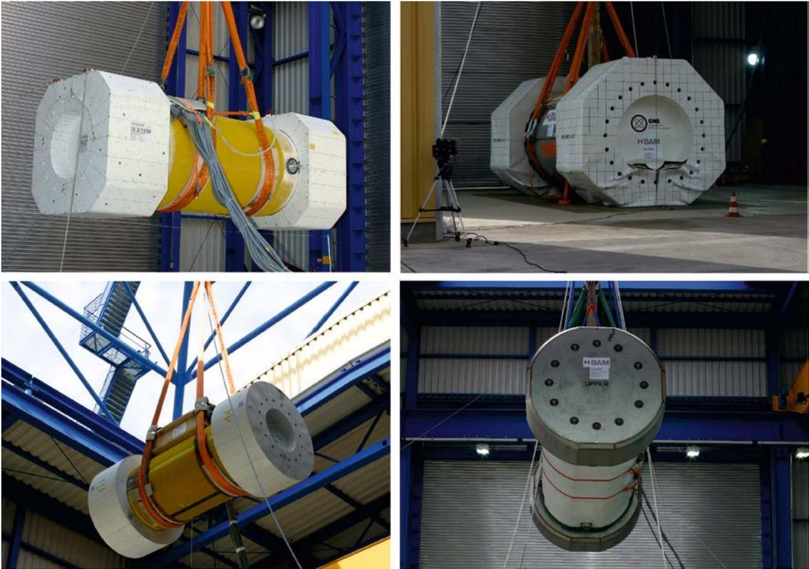
Figure 4. Different impact limiters designs
