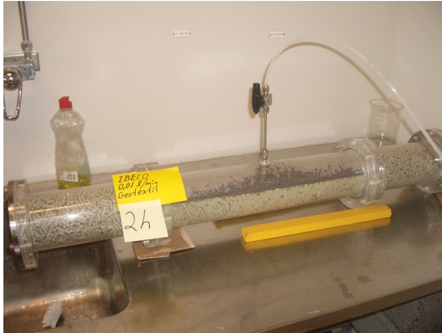
Fig. 2. Picture showing the test equipment used in order to study the function of geotextiles as water distributor.
