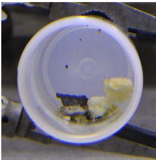
Fig. 5. Sample material collected from the annulus floor near Riser 83.
