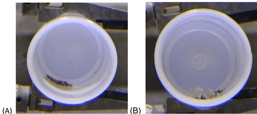
Fig. 7. Samples collected October 17, 2012 from the mound (A) and air-slot (B) locations in the annulus near Riser 90.
