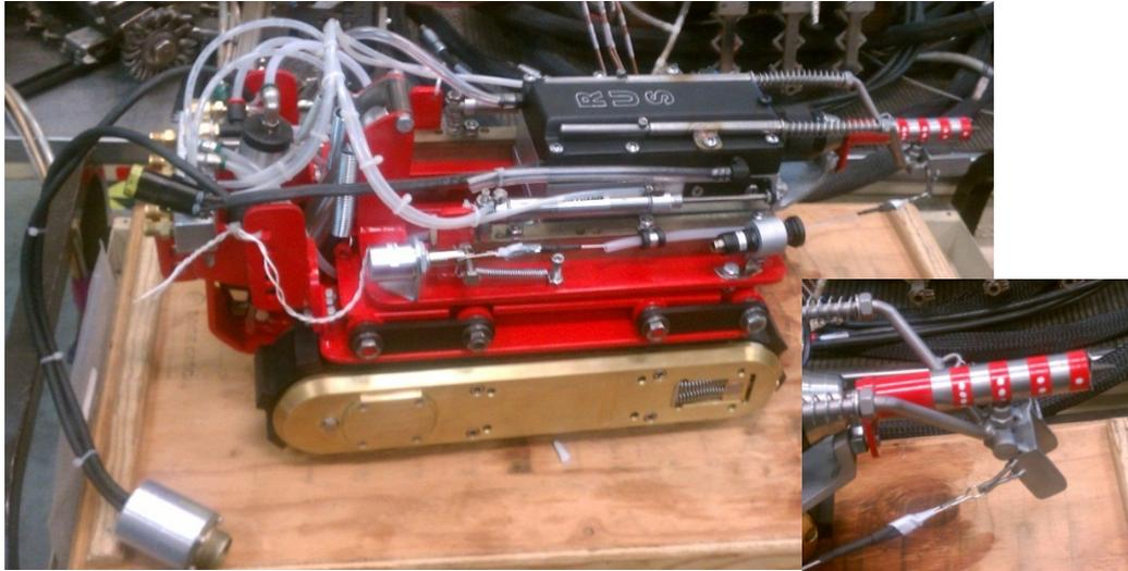
Fig. 3. The Remote Underground Sampler designed to collect material from the annulus sample locations near Riser 90.
