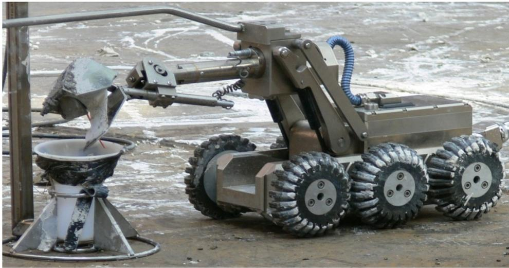
Fig. 2. The Hanford tank farms Off-Riser Sampling System.
