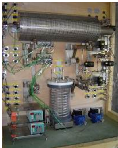
Fig. 10 a and b: Supercritical set-up for separation processes (blank test and oil storage in shielded cell)
