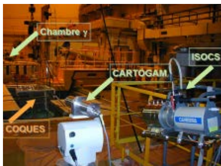
Fig. 6 a and b: Gamma Camera and In Situ Spectrometer System (ISOCS) Gamma probe positioned in UP1 plant
