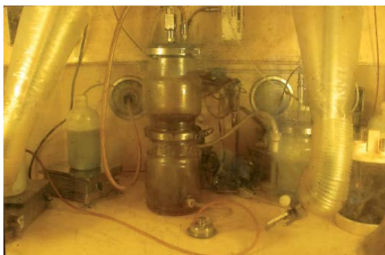
Fig. 10 a and b: Supercritical set-up for separation processes (blank test and oil storage in shielded cell)
