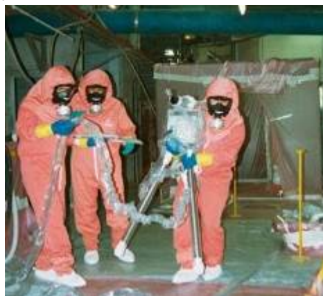
Fig. 6 a and b: Gamma Camera and In Situ Spectrometer System (ISOCS) Gamma probe positioned in UP1 plant
