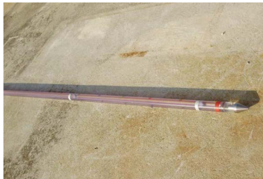
Figure 4. Tube inserted in the sludge
