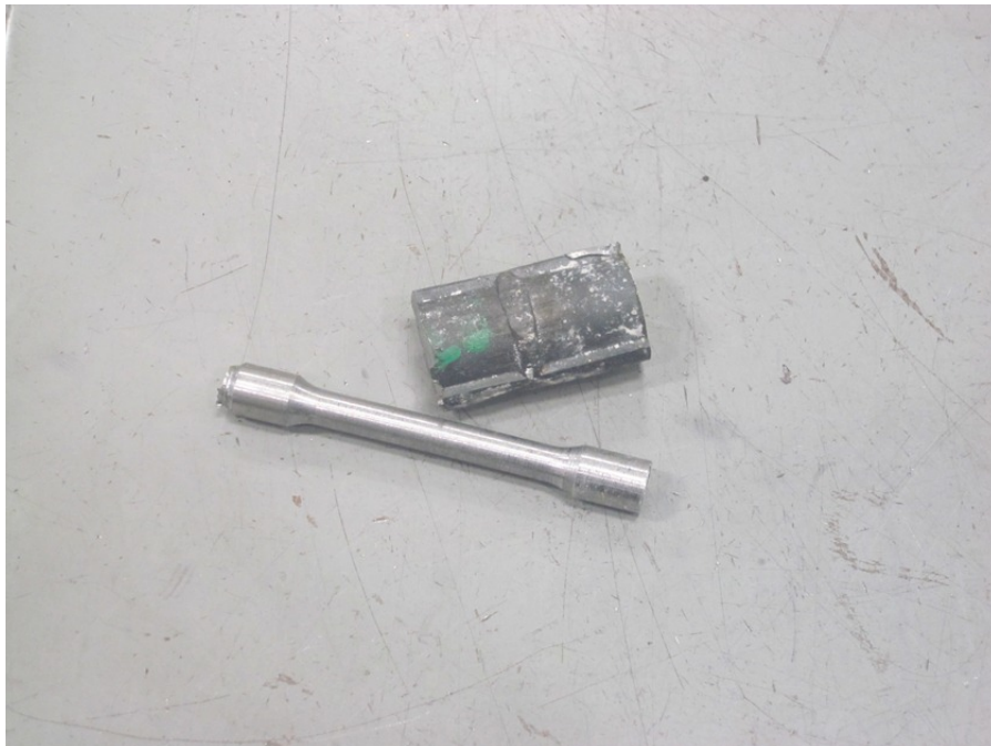
Figure 9. C-107 ASTM A370 Specimen
