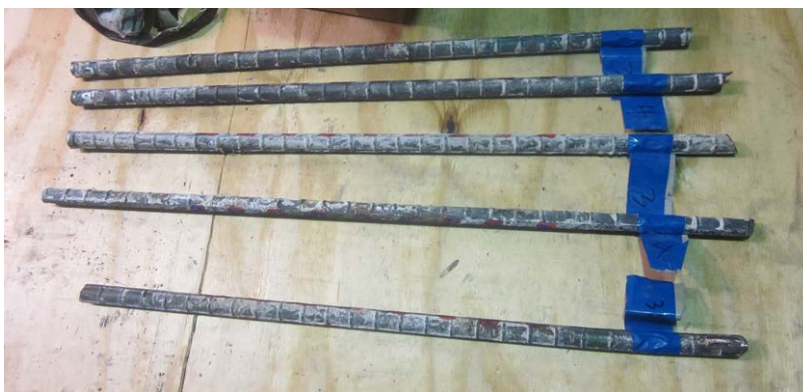
Figure 10. C-107 ASTM A615 Tension Test Specimens
