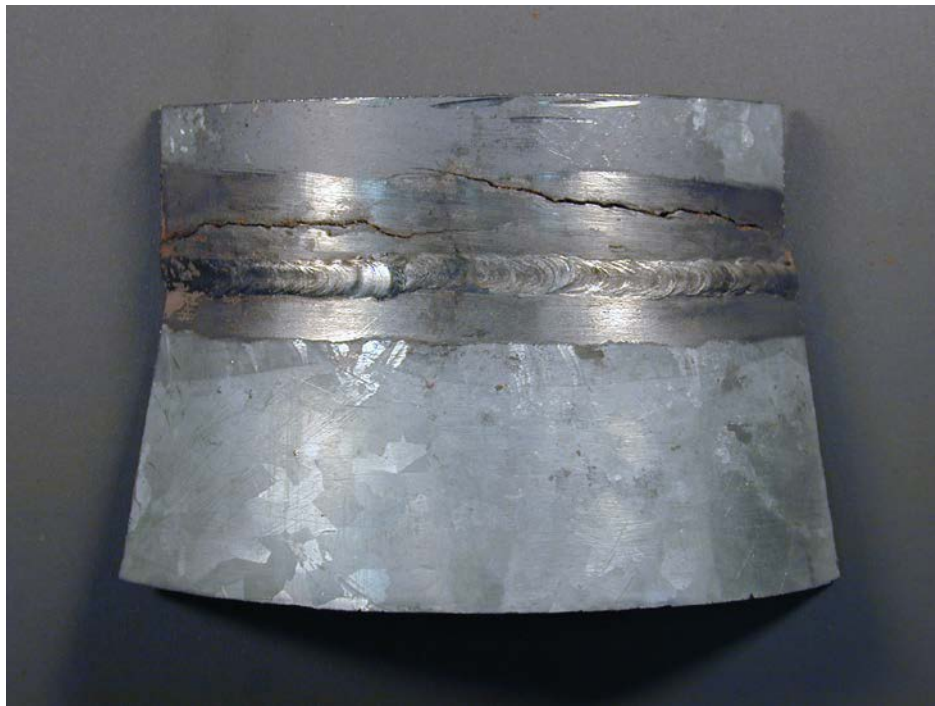
Figure 6. Section of ventilation ductwork removed from the exhaust of the purge ventilation system. Two cracks are evident. A third crack, located on the opposite side of the weld, occurred on the inside surface but did not penetrate to the exterior. Magnification is 1.25 X.
