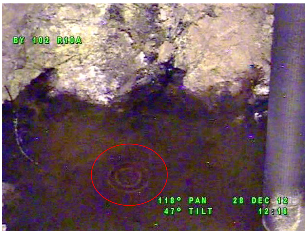
Fig. 2. Tank BY-102 ripples in liquid pool.
