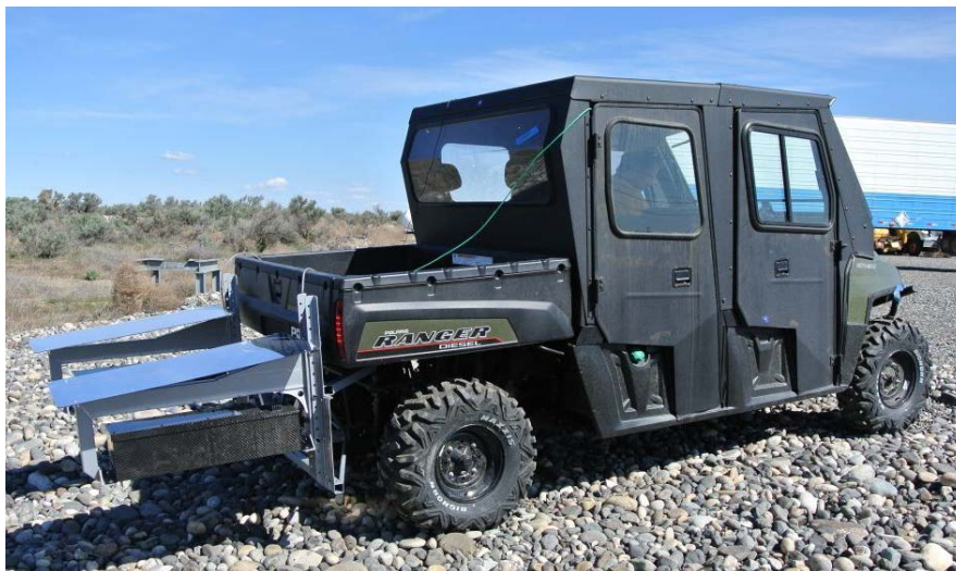
The mobile gamma spectrometer is mounted on a Polaris all-terrain vehicle.
