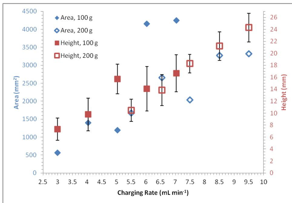
Fig. 2. Cold-cap height and area, prepared with 100- or 200-g initial glass, versus charging rate
