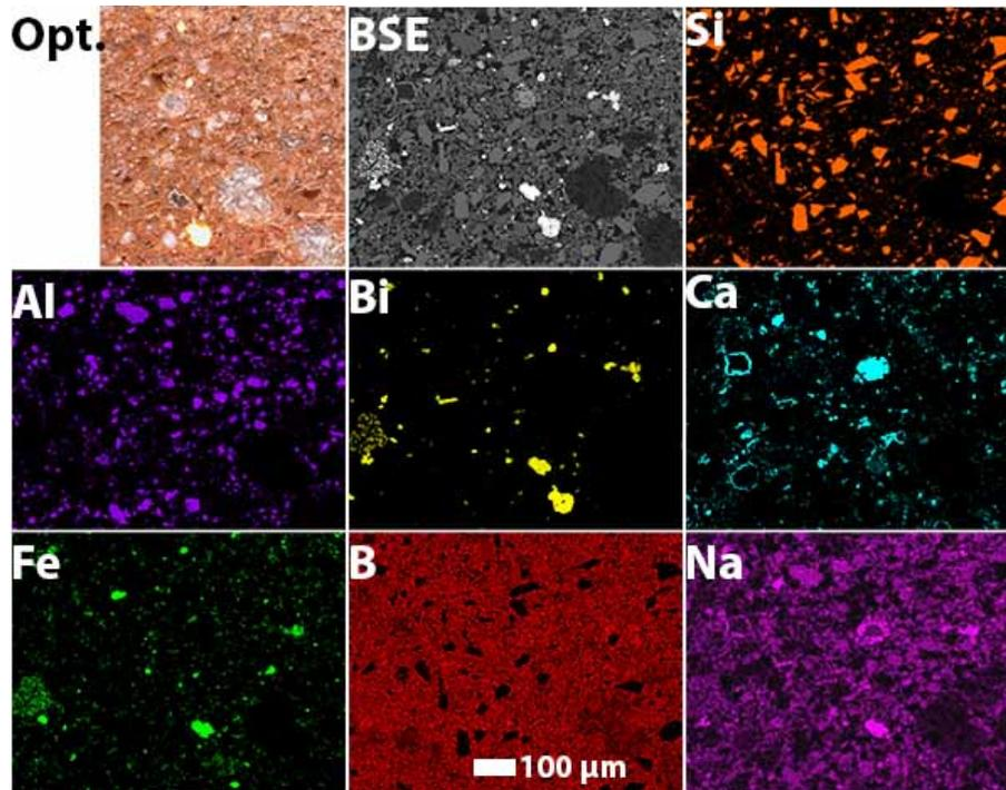
Fig. 7. Elemental map of a region near the top of the cold cap as shown by the blue box shown in Fig. 3
