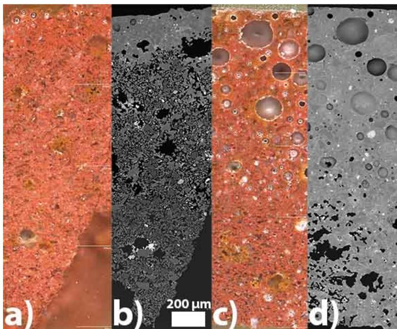
Fig. 6. Optical [a) and c)] and BSE [b) and d)] images of heat-treated A0 feed at 5 K min<sup>-1</sup> to 700 [a) and b)] 800°C [c) and d)]
