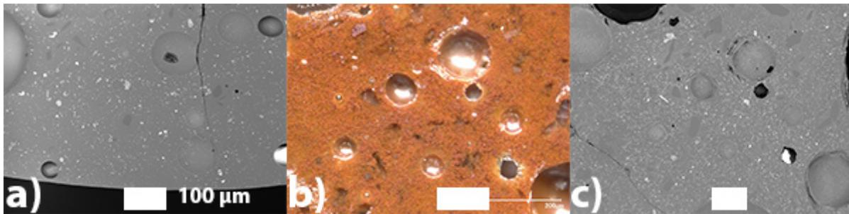
Fig. 5. a) BSE micrograph of heat-treated A0 feed at 900°C. A similarly structured region of the cold cap was found at the location of the marked red box in Fig. 3, as seen in images of an identical region from optical microscopy (image 5b) and BSE micrographs (5c).
