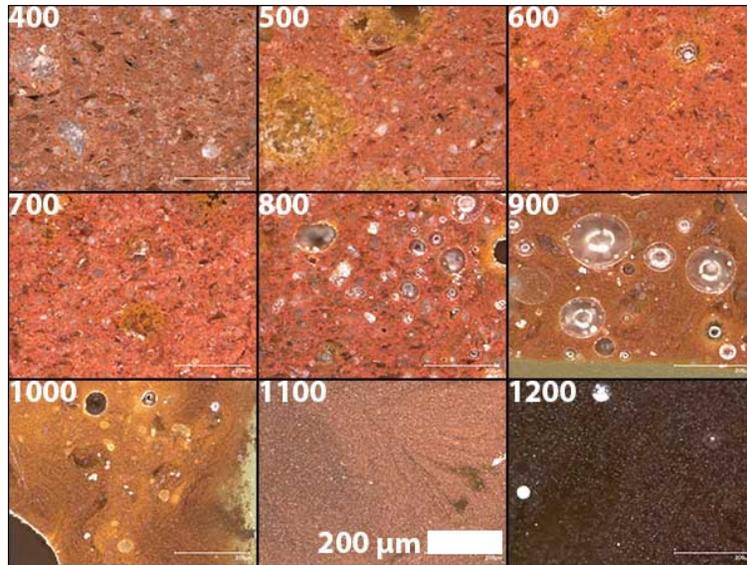
Fig. 4. Matrix of heat-treated samples of A0 composition. All temperatures are in units of °C, and all size bars denote 200 µm.
