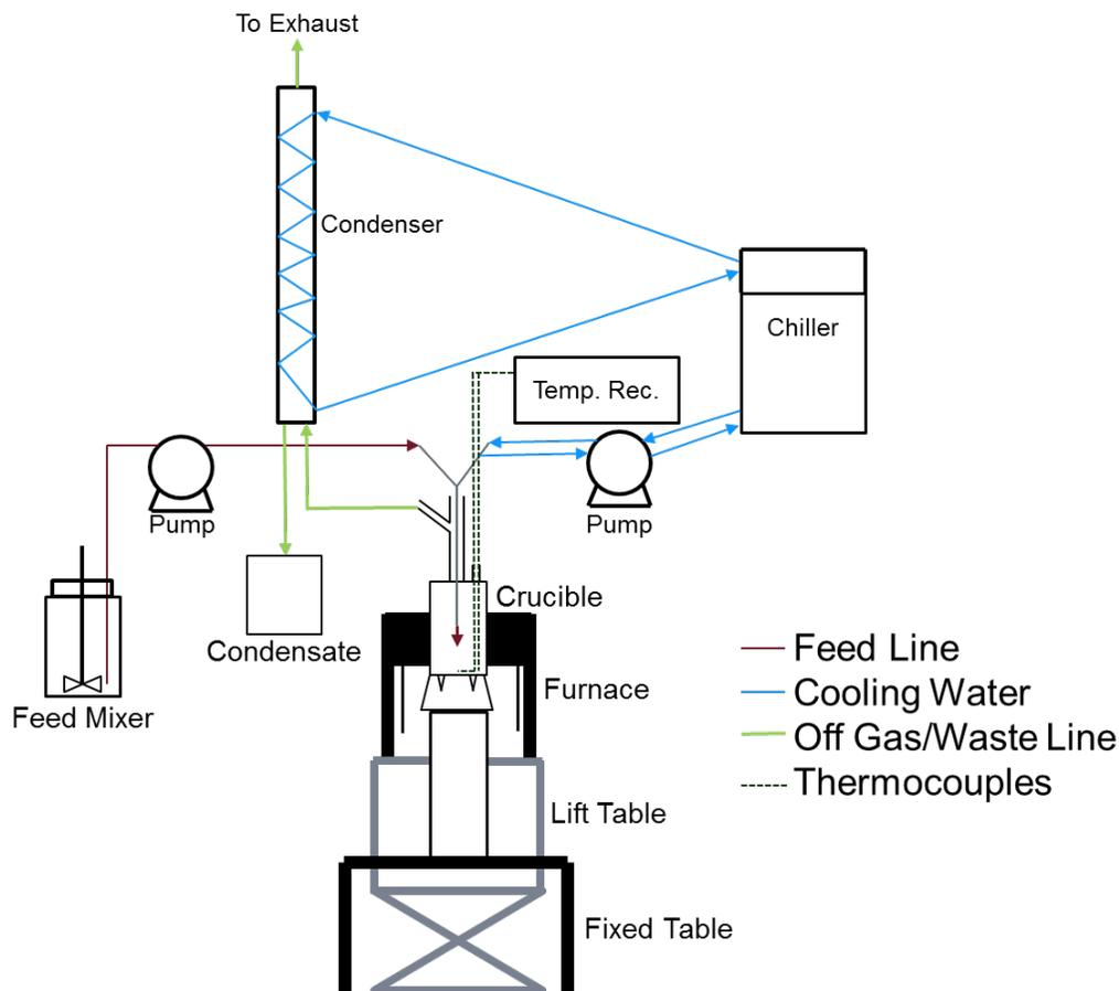
Fig. 1. Schematic of the LSM system. The pump on the left charges slurry feed into the crucible, and the pump on the right circulates cooling water from the chiller to the feed injection nozzle and back.
