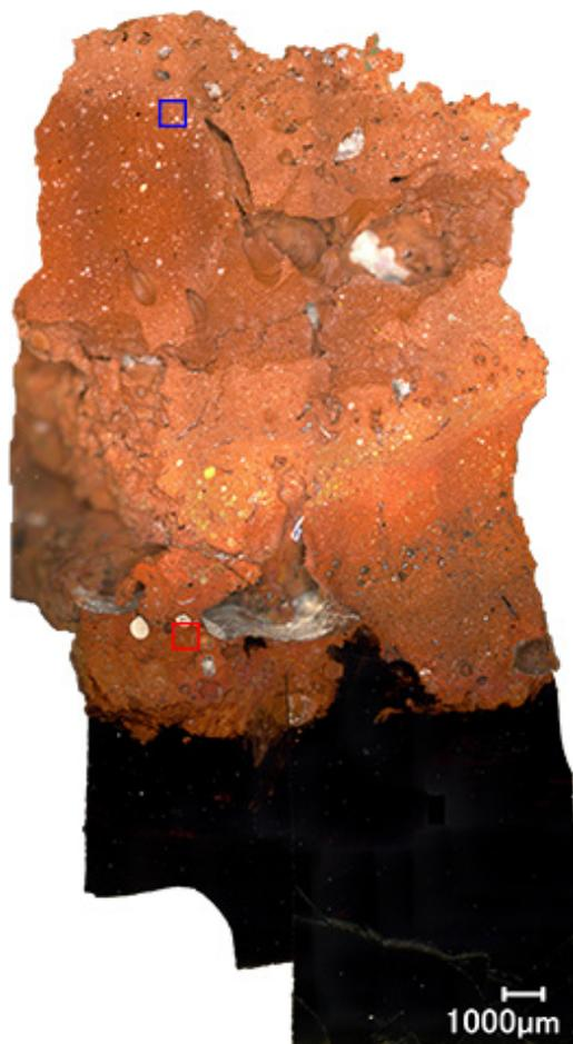
Fig. 3. Polished cold-cap cross section from the 6.5 mL min<sup>-1</sup> run. Regions for further analysis are marked by the blue (top of sample) and red boxes.
