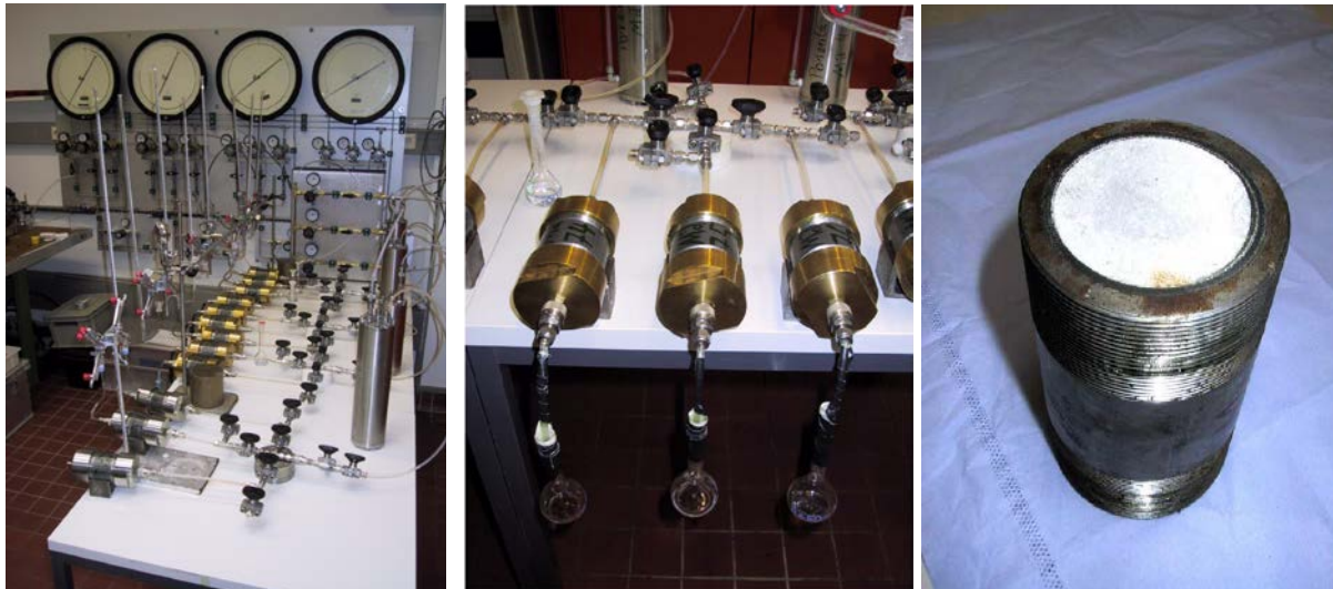
Fig. 7 Photograph of the experimental set-up for measurements of corrosion progress and permeability changes during the interaction of brines with concretes [2]
