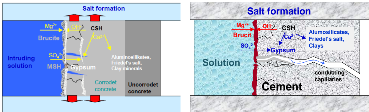
Fig. 2 Schematic representation of the chemical corrosion processes in salt concrete due to the interaction with Mg-, SO 4 and Cl-rich salt solutions (left) diffusive matrix corrosion, (right) advective corrosion on cracks (in [1] modified after [2])
