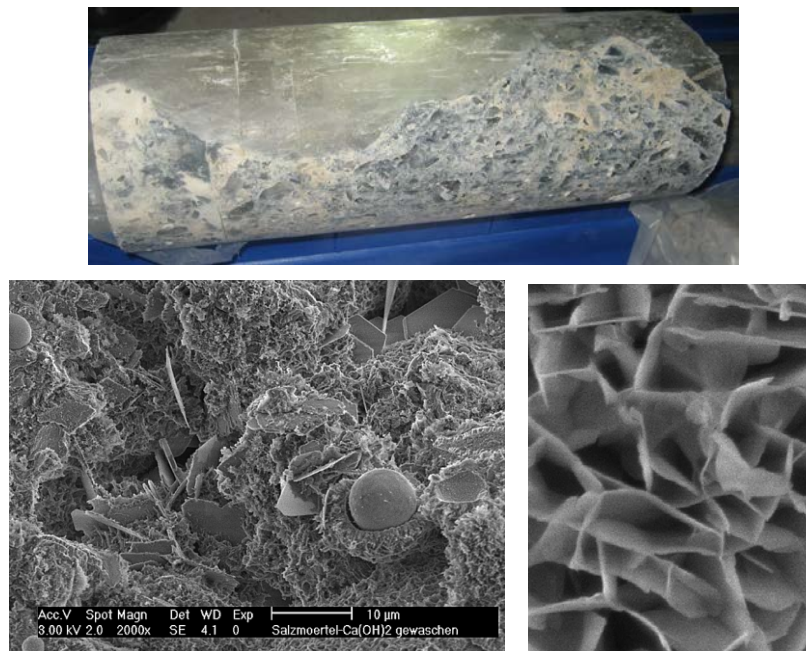
Fig. 3 (above) Salt concrete in contact with salt – core form the contact of a salt concrete seal in the Asse mine; (below left) CSH-phases in salt concrete covered by halite; Friedels salt (hexagonal plates); (below right) CSH phases
