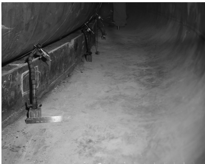
Fig. 4. Strain gage monitoring in tank SY-103 to assess impacts from primary bottom bulges.
