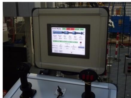
Figure 5 - Operator Control Unit
