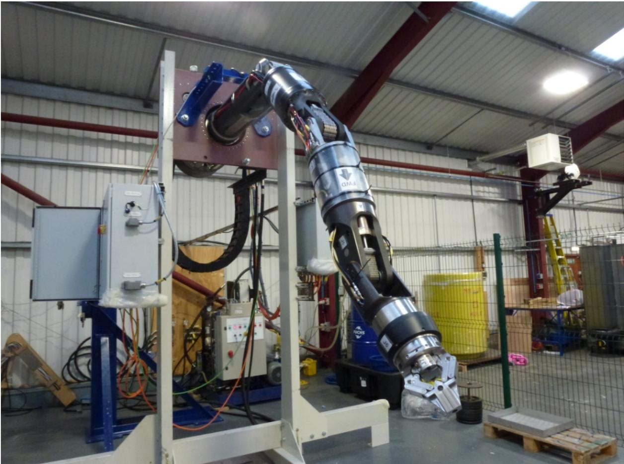
**Figure 1 - Prototype ModuMan during Factory Acceptance Testing**
