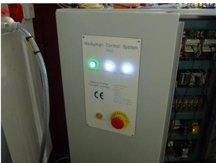
Figure 4 - Control Console Unit
