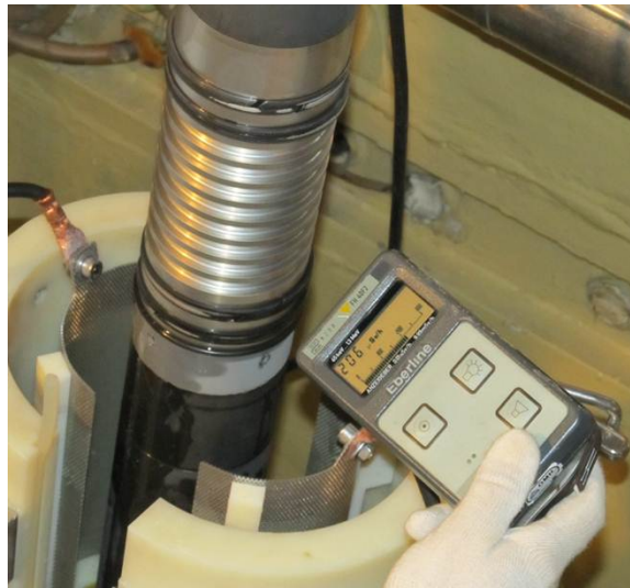
Figure 5. Dose measurement during the decontamination of the labyrinth threads
