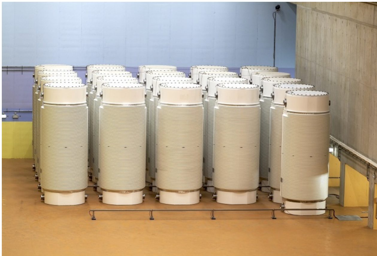
Figure 1: CASTOR® V casks in storage on-site at the German nuclear power station Emsland
