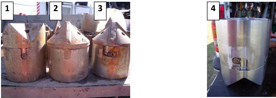
Figure 7 - Locking Mechanism Development: 1) Push-lock with shim, 2) welded onto drive shoe, 3 & 4) twist lock with pin
