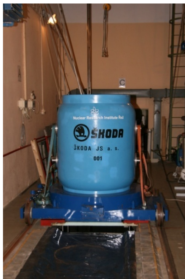
Fig. 3. ŠKODA VPVR/M cask prepared for loading onto the storage pool
