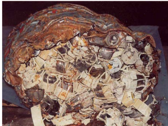
Fig. 8: Example of a drum with ionizing fire detector seized in the scrap yard
