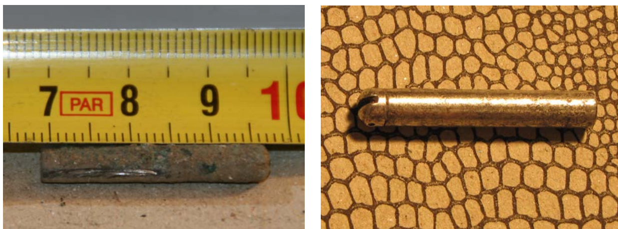
Fig. 5: Size of removed source and how it looks like before and after cleaning
