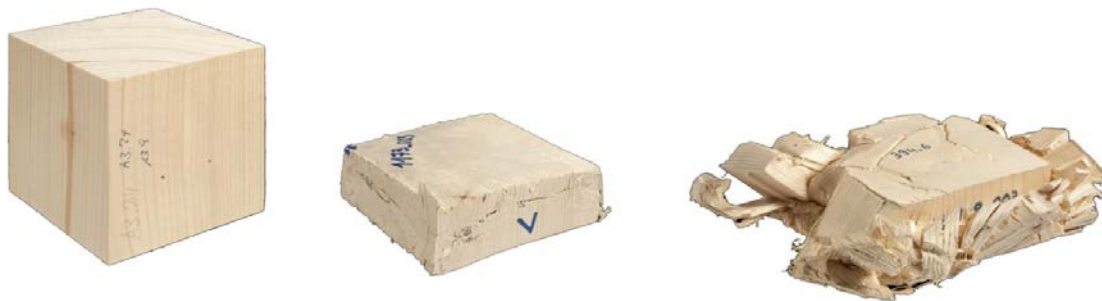
Figure 2. Spruce wood specimen before the crush test (lhs). Specimen loaded parallel to the fiber crushed with (middle) and without lateral constraint (rhs).
