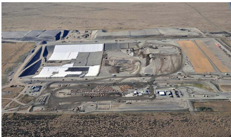
Fig. 1. Environmental Restoration Disposal Facility at Hanford during construction of liner and leachate system for new cells (DOE Photo).
