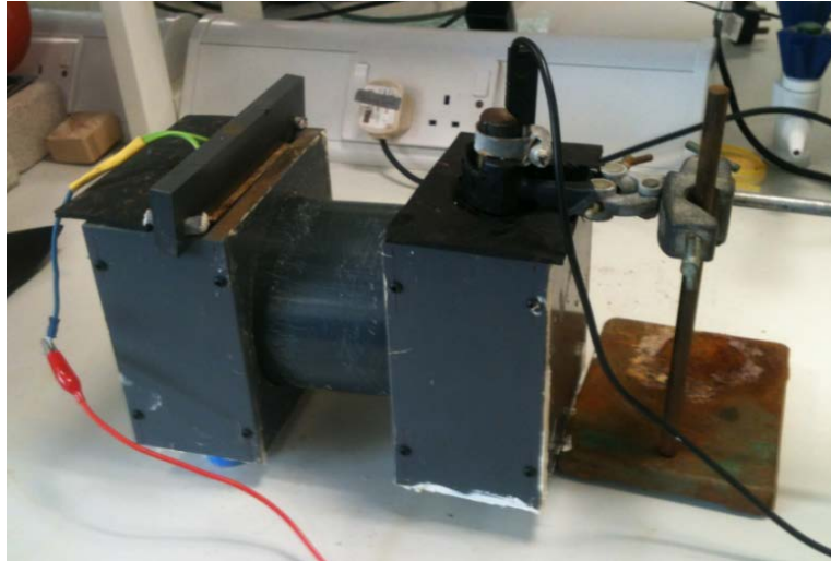
Figure 1. The analytical phantom, housing the concrete sample between the anode compartment, left, and the cathode compartment, right.
