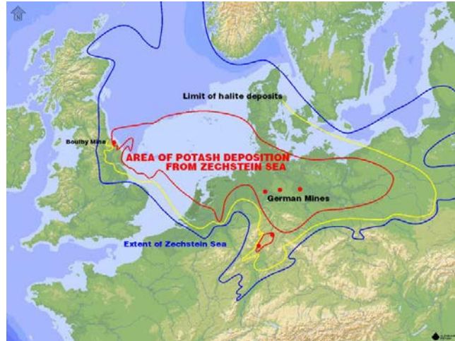
Fig. 2. Potentially suitable salt formations in the north-western part of Europe including the North Sea. The red area is of potential interest [10].
