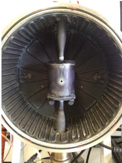
Figure 2. Hot uniaxial press and furnace used in initial testing for \text{Ag}^0\text{Z} pressing.
