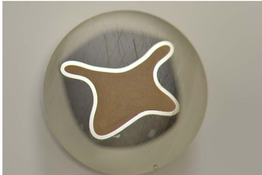
Figure 12. Cross section of HIPed sample 2 (700°C and 100 MPa).
