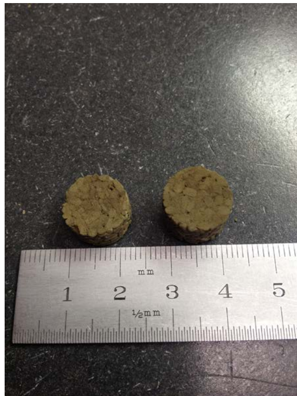
Figure 5. Cross section of HUPed compact from pellet form \text{Ag}^0\text{Z} .
