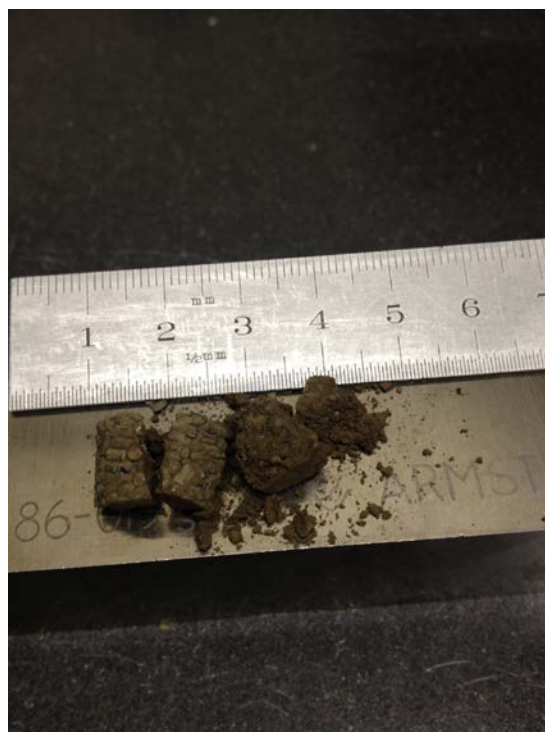
Figure 6. Crushed HUPed compact formed from pellet form \text{Ag}^0\text{Z} .
