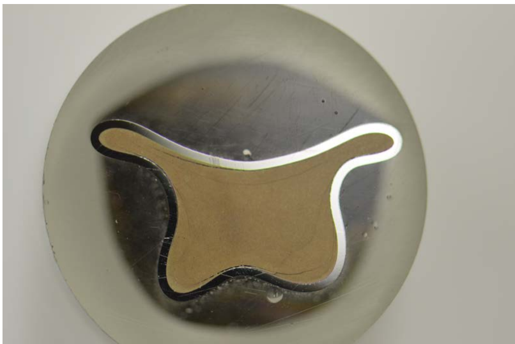
Figure 14. Cross section of HIPed sample 6 (crushed AgZ, 700°C and 100 MPa).
