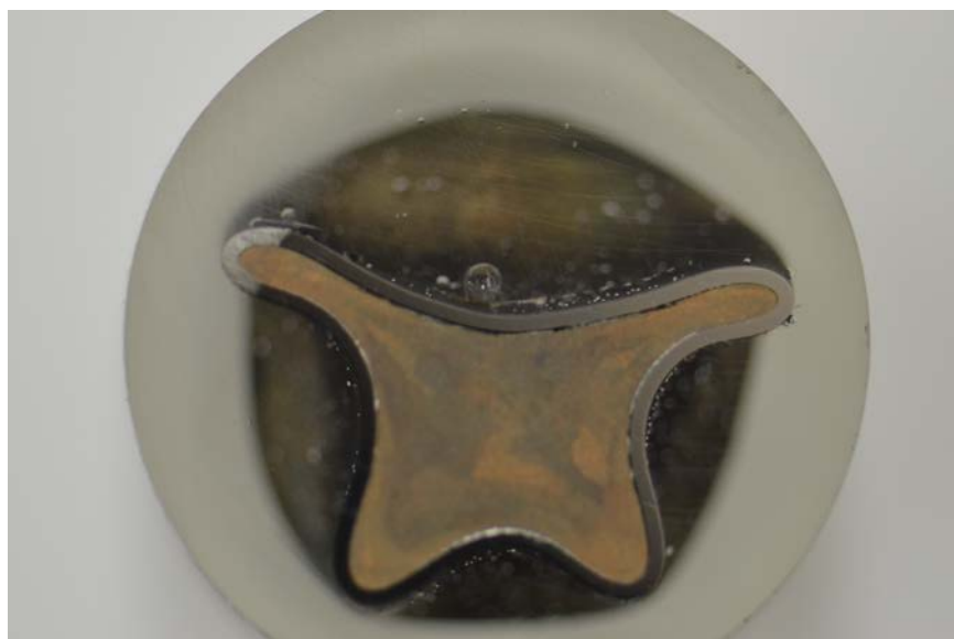
Figure 15. Cross section of HIPed sample 8 containing I-AgZ (700°C and 175 MPa).
