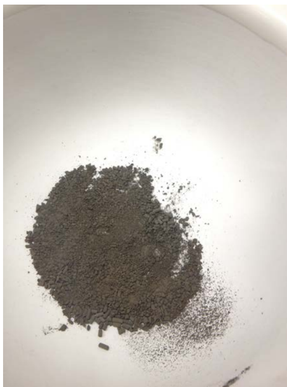
Figure 1. Crushed Ag 0 Z used in HUP testing.
