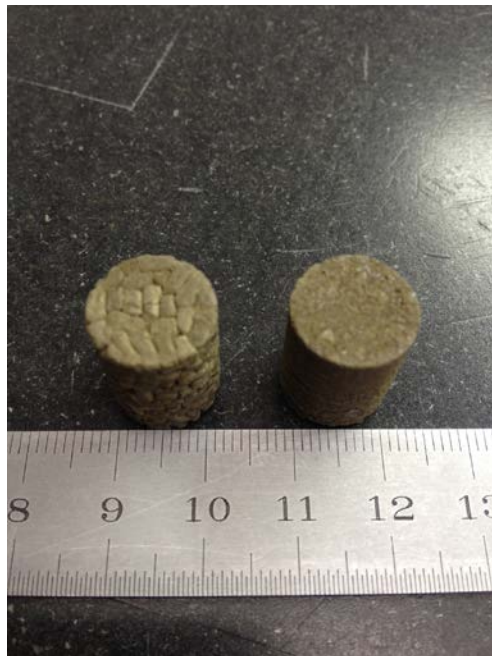
Figure 3. HUPed compacts from pellet form \text{Ag}^0\text{Z} (left) and crushed \text{Ag}^0\text{Z} (right).
