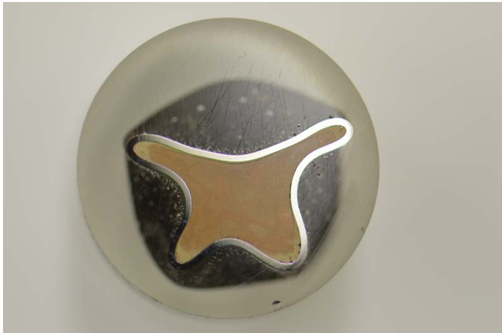
Figure 13. Cross section of HIPed sample 3 (700°C and 175 MPa).
