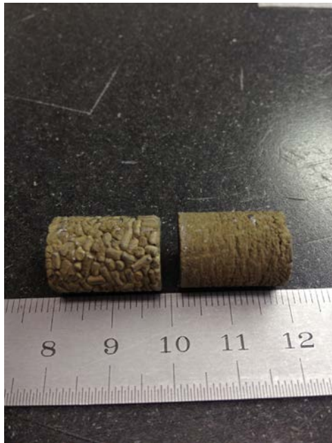
Figure 4. Side view of HUPed compacts from pellet form \text{Ag}^0\text{Z} (left) and crushed \text{Ag}^0\text{Z} (right).
