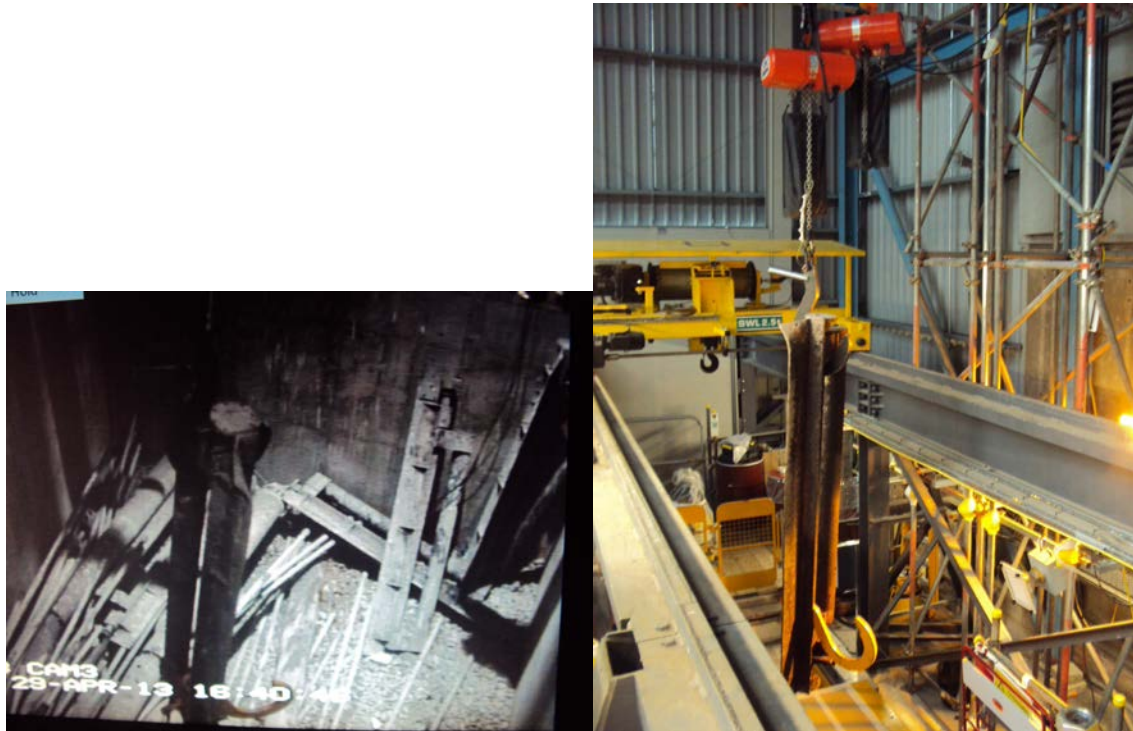
Figure 5: ‘Lost’ hook retrieving with waste (bomb door) using secondary equipment.
