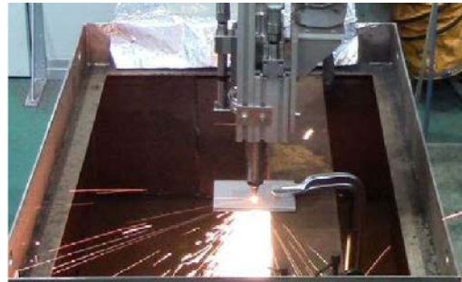
Figure 4: Example of the cut test pieces for 10 mm thickness stainless steel plate (Laser Power: 3kW, Cutting Speed: 500 mm/min)
