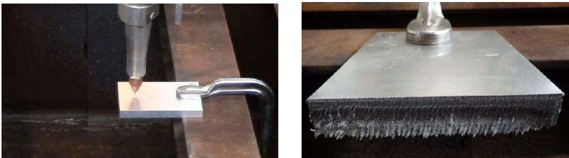
Figure 9: The laser cutting for aluminum alloy of 10 mm in thickness (Laser Power: 5 kW, Cutting Speed: 250 mm/min)
