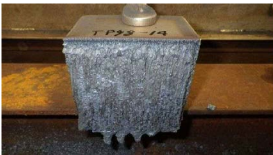
Figure 5: Example of the cut test pieces for 100 mm thickness stainless steel plate (Laser Power: 9kW, Cutting Speed: 30 mm/min)
