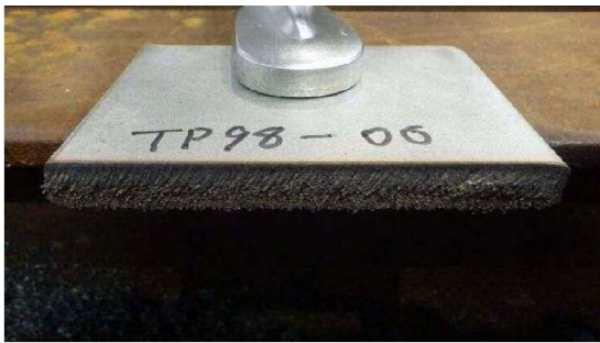
Figure 4: Example of the cut test pieces for 10 mm thickness stainless steel plate (Laser Power: 3kW, Cutting Speed: 500 mm/min)
