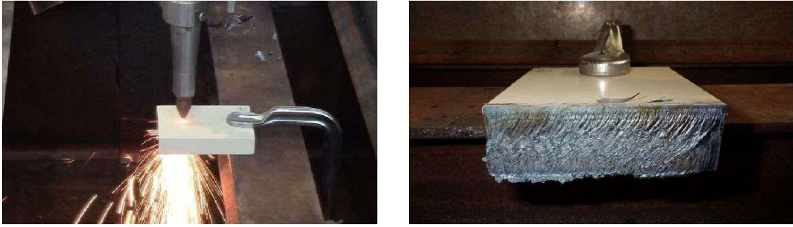
Figure 8: The laser cutting for painted steel of 30 mm in thickness (Laser Power: 6 kW, Cutting Speed: 190 mm/min)
