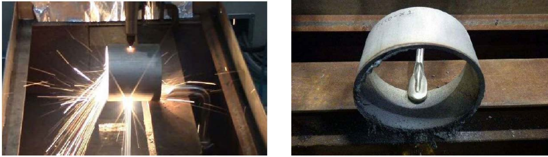
Figure 11: The laser cutting for stainless steel pipe ( \phi 165.2 mm and t = 5 mm, Laser power: 9 kW, Cutting Speed: 100 mm/min)
