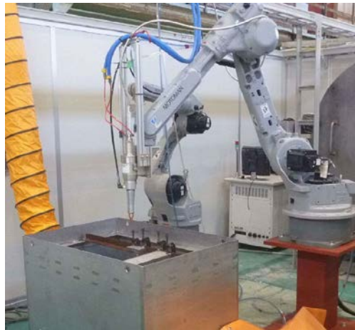
Figure 3: Equipment for the laser cutting tests
