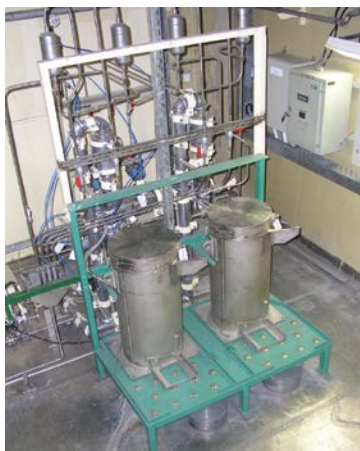
Fig. 2. The ion exchange column and the shielding system
