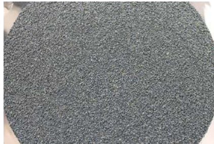
Fig.4. CsFix cesium selective sorbent
