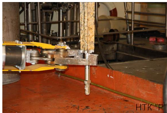
Fig.4. Separation of aluminum shaft from the beryllium block
