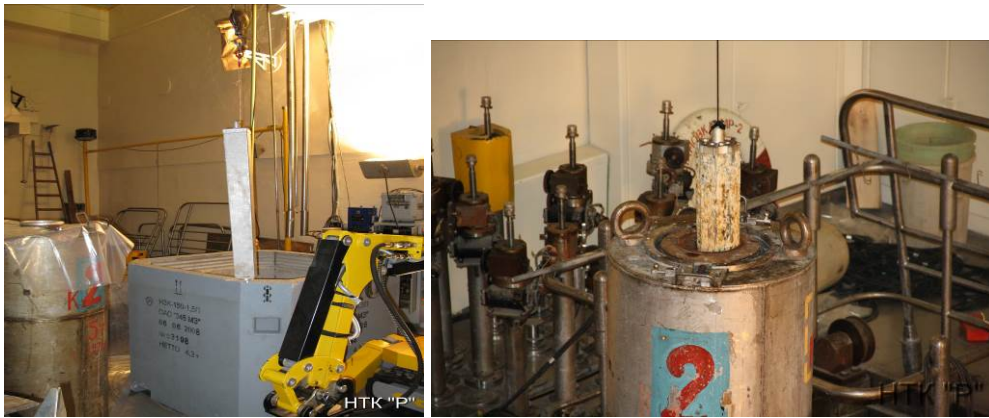
Fig. 5. Loading of radwaste in transport and lead containers
