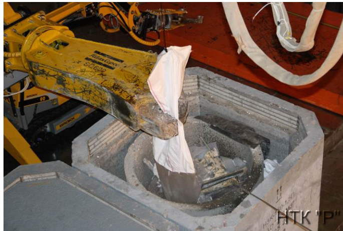
Fig. 7. Fragmentation of high active beryllium blocks and loading them into NZK-150-1.5P container.
