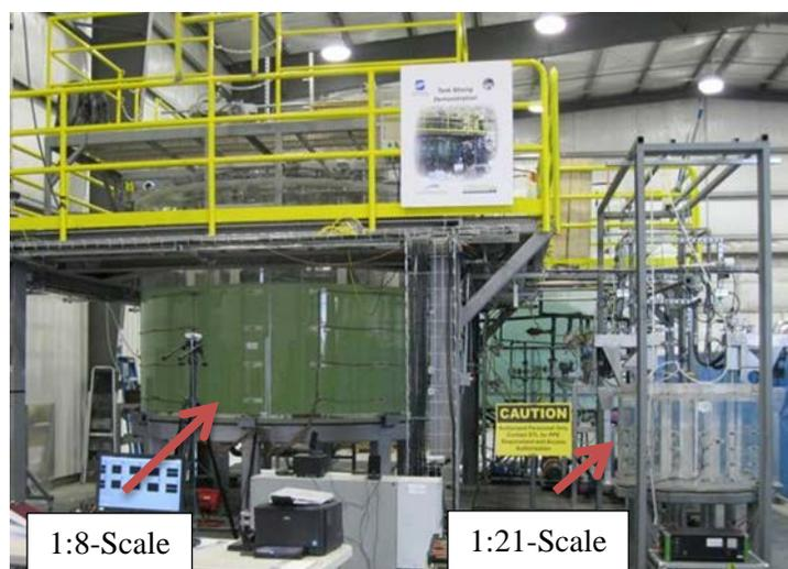
Figure 1. Small-scale mixing demonstration test platform
