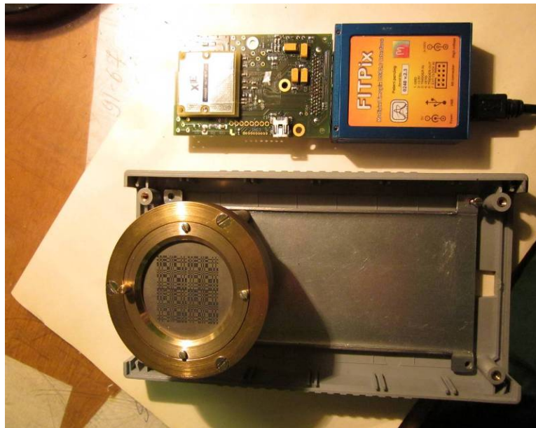
Figure 4. Detector Medipix2 with communication module FITPix before installing into the detector housing with block of coded mask
