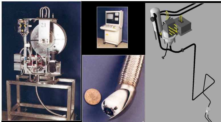
Fig. 7. Pipe Unblocking Equipment
