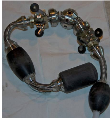
Fig. 4. Coil Inspection Device
