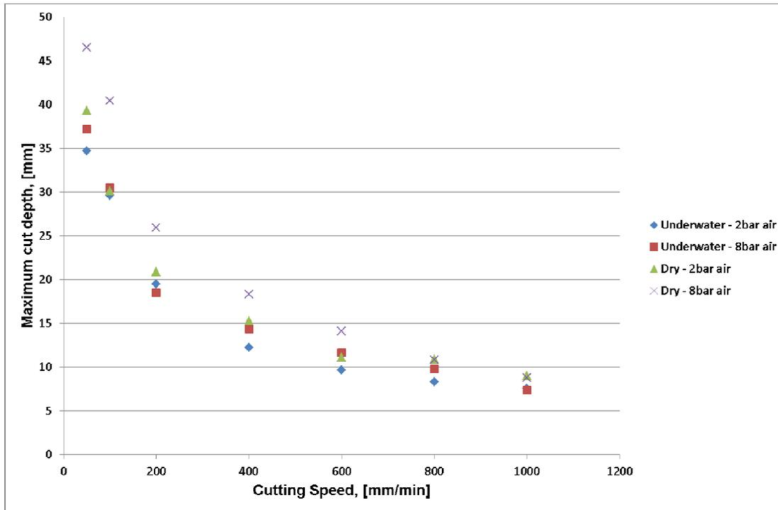
**Fig. 2.** Maximum cut depths achieved for the underwater and in-air cutting processes as a function of cutting speed using 2 and 8bar coaxial assist gas pressures, using 4.8kW of laser power with a standoff distance of 15mm.
