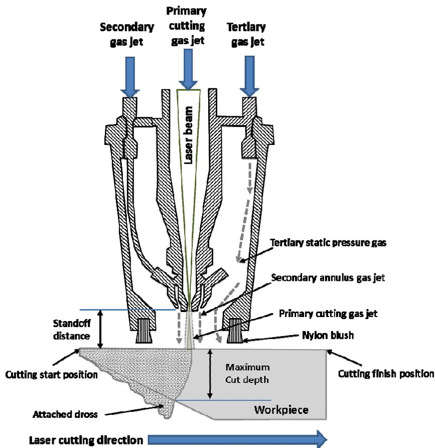
Fig. 1. Underwater laser cutting process schematic.
