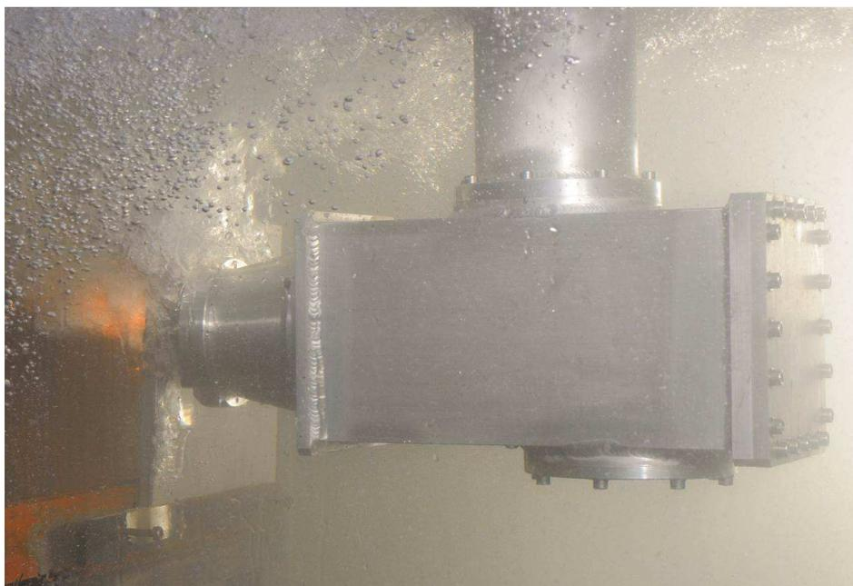
**Fig. 5.** The underwater laser cutting unit in operation.
