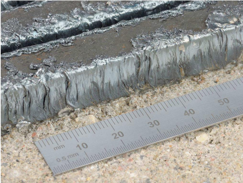
**Fig. 9.** Gouge cutting of 12mm thickness CMn steel on top of concrete, with minimum damage to the concrete surface.
