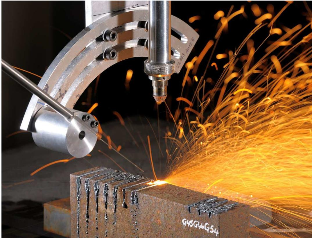
**Fig. 6.** The lower end of the gouge cutting head, showing the conventional co-axial assist gas/beam delivery nozzle and the side gas-jet. In this case the side gas is delivered through a narrow stainless steel tube so that, as successive cuts are made, the end of this nozzle can descend into the cutting groove.
