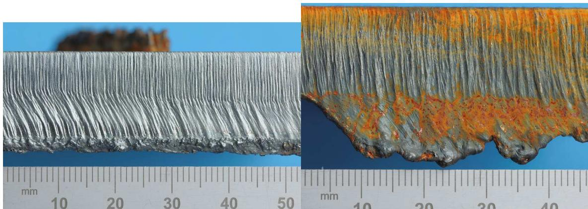
**Fig. 3.** Edges of 15mm S355 C-Mn steel plate cut underwater (right) and in-air (left) at the parameters described in the text.
