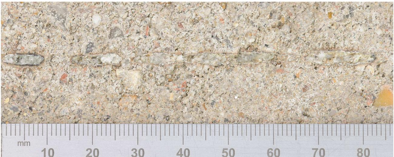
**Fig. 10.** Effect on the concrete surface after removal of the steel.
