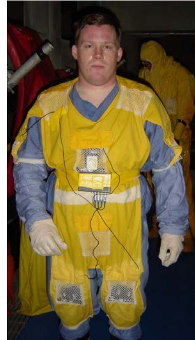
Fig. 6. Teledosimetry is worn under the diver's dry suit.
