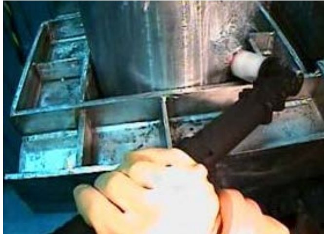
Fig. 7. Plasma torch cutting head in use by diver.
