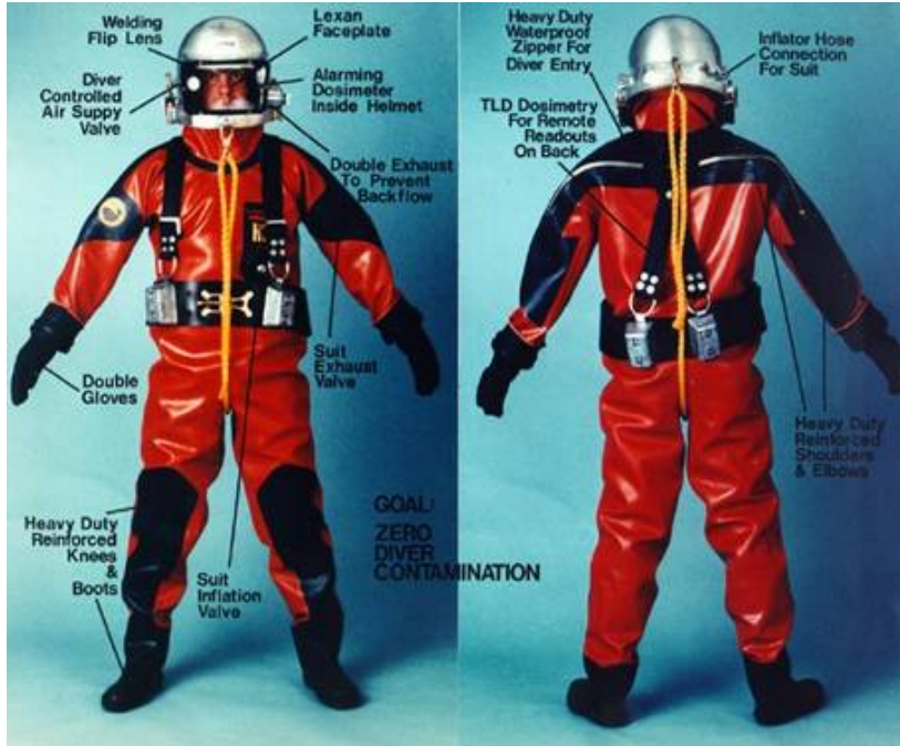
Fig. 5. Typical dive equipment configuration for contaminated diving operations.
