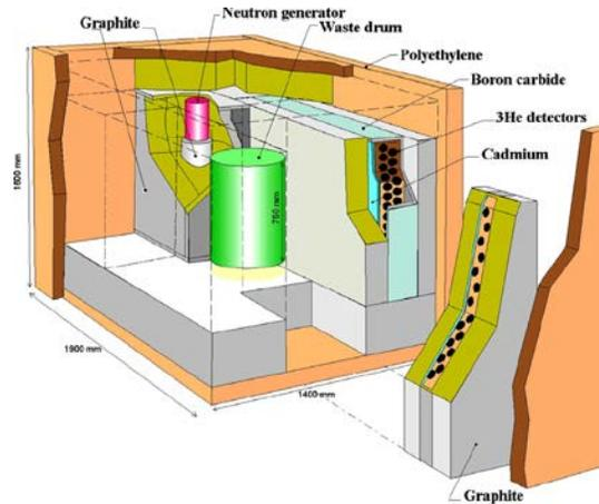
Fig. 1. Schematic view of the PROMETHEE 6 measurement cell.
