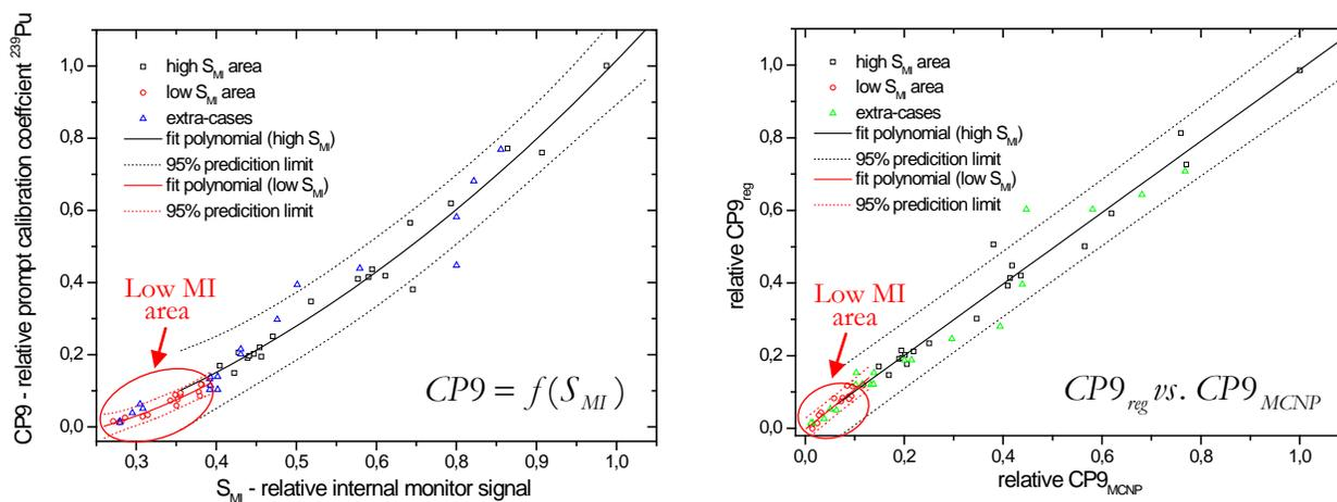
Fig. 6. a) Correlation between the prompt neutron calibration coefficient and the internal monitor signal  $S_{MI}$  b) Relationship between the predicted CP9 (i.e.  $CP9_{reg}$ ) and the one calculated, with MCNP (the objective being closer to  $CP9_{reg}=CP9_{MCNP}$ ). Both  $S_{MI}$  and  $CP9$  are normalized to their maximal values.
