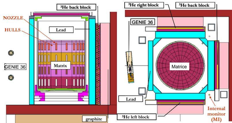
Fig. 4. MCNP plots of P0-2 measurement cell showing 800 litres drum and the internal monitor (MI)
