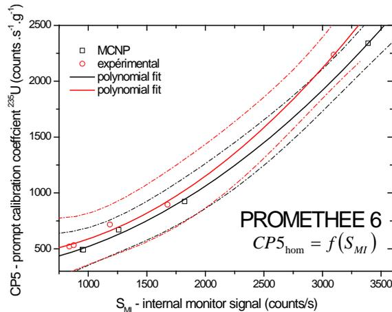
Fig. 2. Relationship between the prompt neutron calibration coefficient for an homogeneous fissile material distribution  $CP5_{\text{hom}}$  and the internal monitor mean signal  $S_{MI}$  for both experiment and MCNP calculation with PROMETHEE 6, from reference [1].
