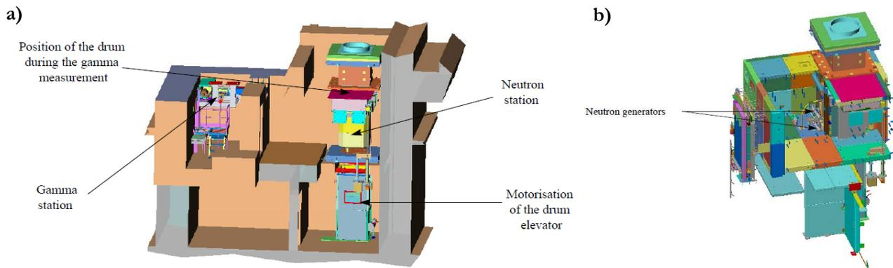
Fig. 3. a) general layout of the incoming measurement station on ACC compacting facility b) layout of the P0-2 measurement cell [10]
