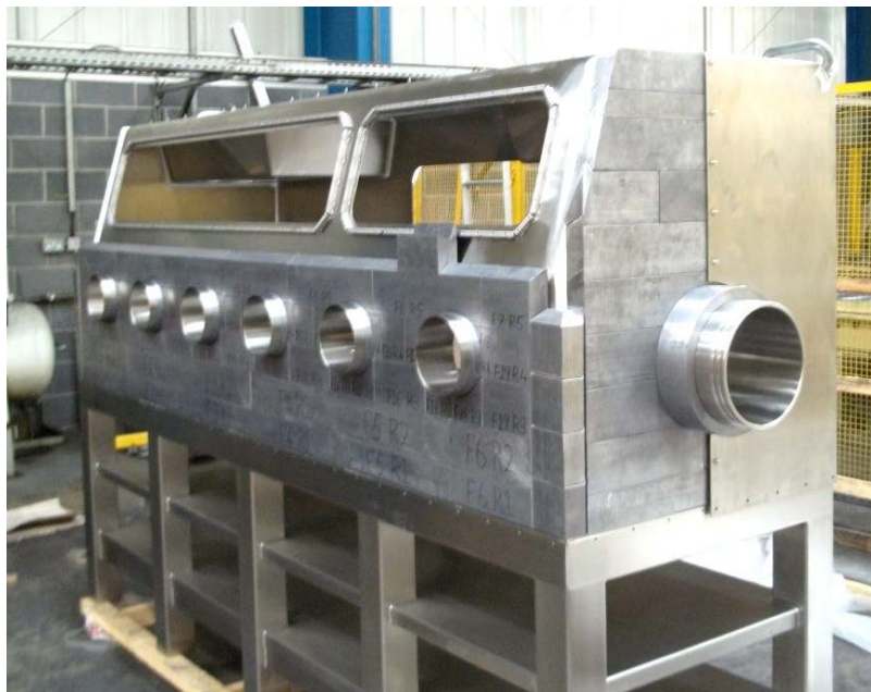
Fig. 8. Hosokawa Lead Shielded Glovebox During Assembly
