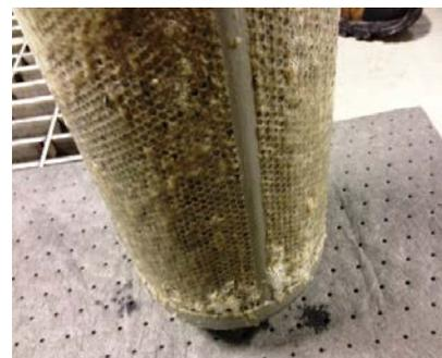
Fig. 2. Biofilm fouling of a straining apparatus.
