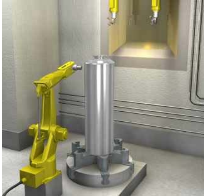
Fig. 2: Inspecting a high-level waste package. © Andra
