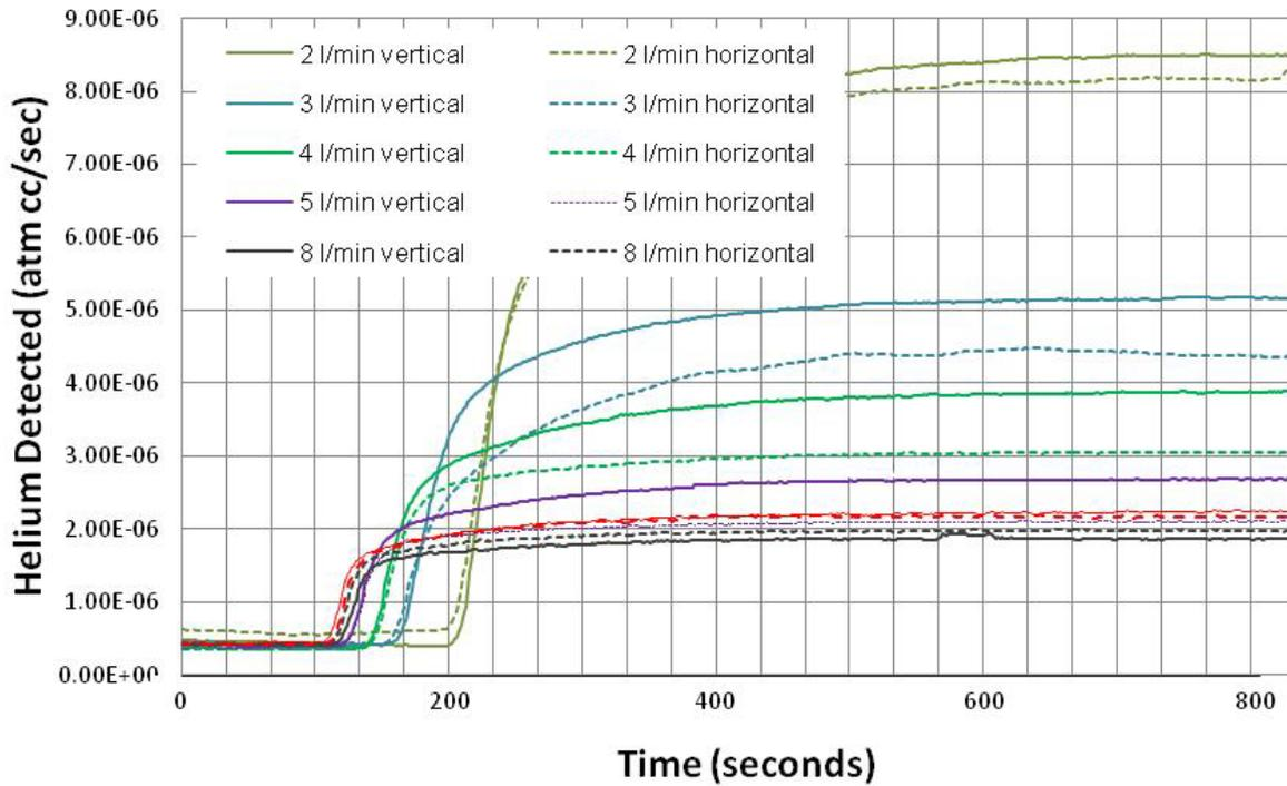
Fig. 2 Helium Detected Following Flow Switch for Various Flow Rates and Tube Orientations
