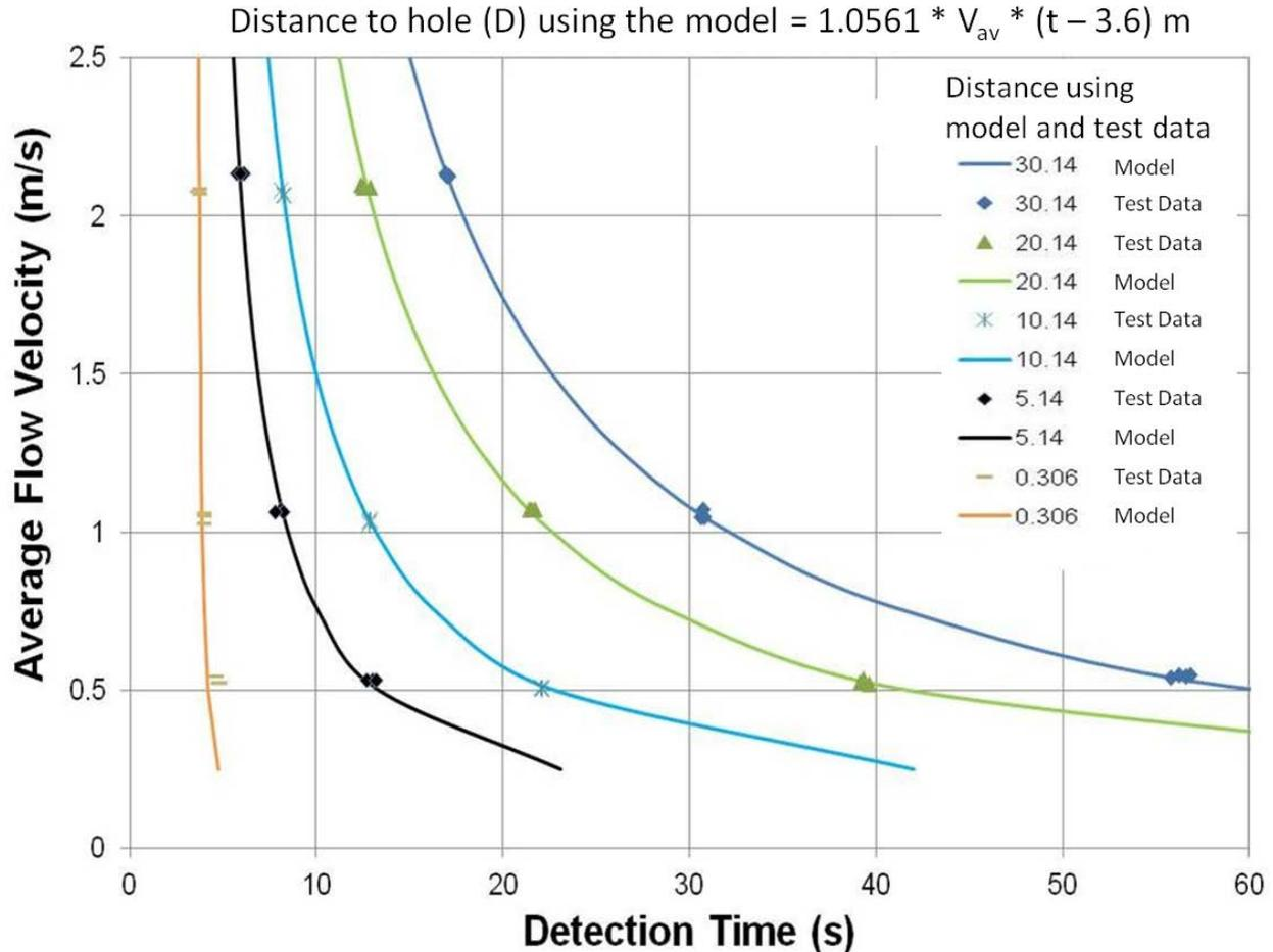
Fig. 5 Average Flow Velocity versus Detection Time for Various Hole Distances and Flow Rates
