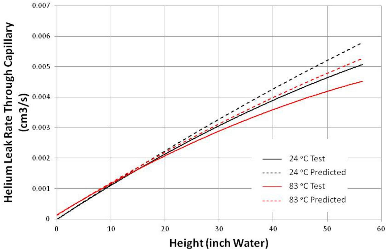
Fig. 8 Comparison of Measured and Predicted Helium Leak Rate at Two Temperatures
