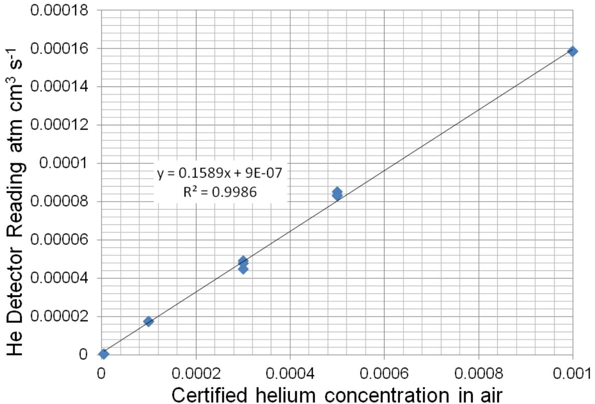
Fig. 6 Correlation of Calibrated Mixtures of He in Air with Helium Detector Readings
