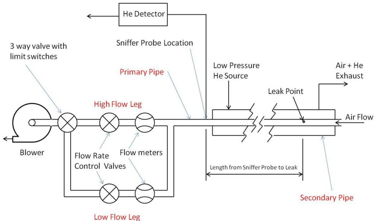
Fig. 4 Schematic Showing Test Apparatus for Determining Leakage Location
