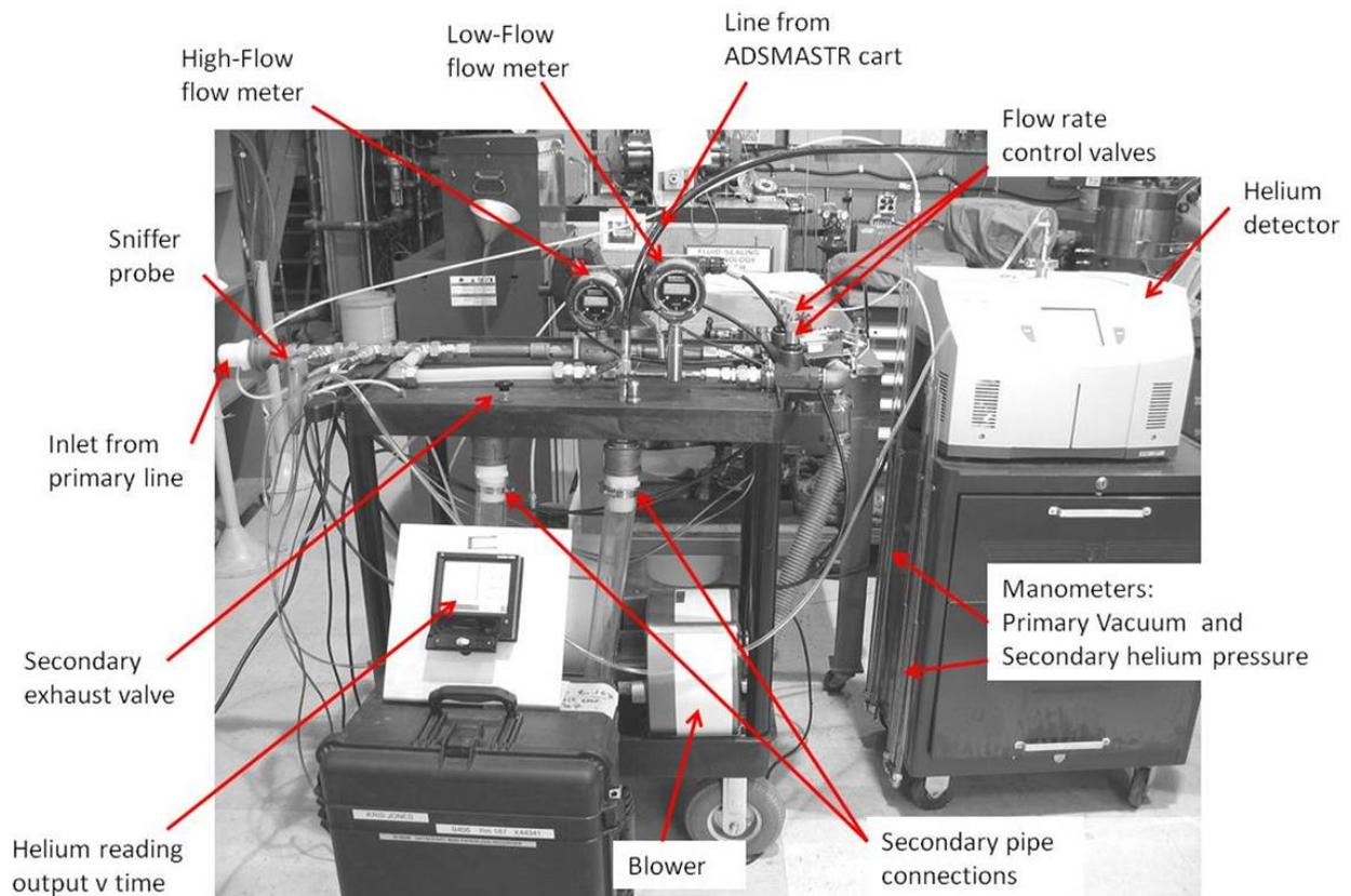
Fig. 9 Portable Equipment used for LLoDS Testing
