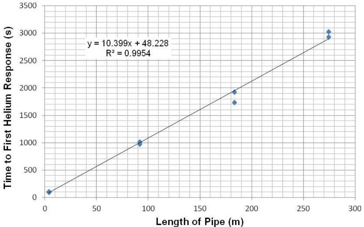
Fig. 3 Helium Detection over Long Lengths of Tubing
