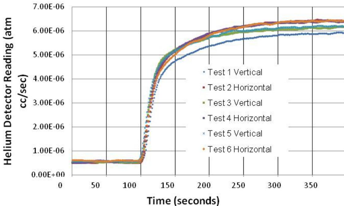
Fig. 1 Helium Detection in Horizontal and Vertical Orientation using 3 m long Tube
