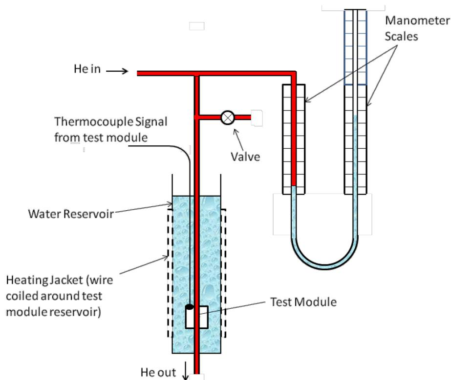
Fig. 7 Schematic of Helium Leak Test Equipment
